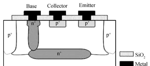
Fig. 1. Schematic cross section of lateral PNP transistors.
