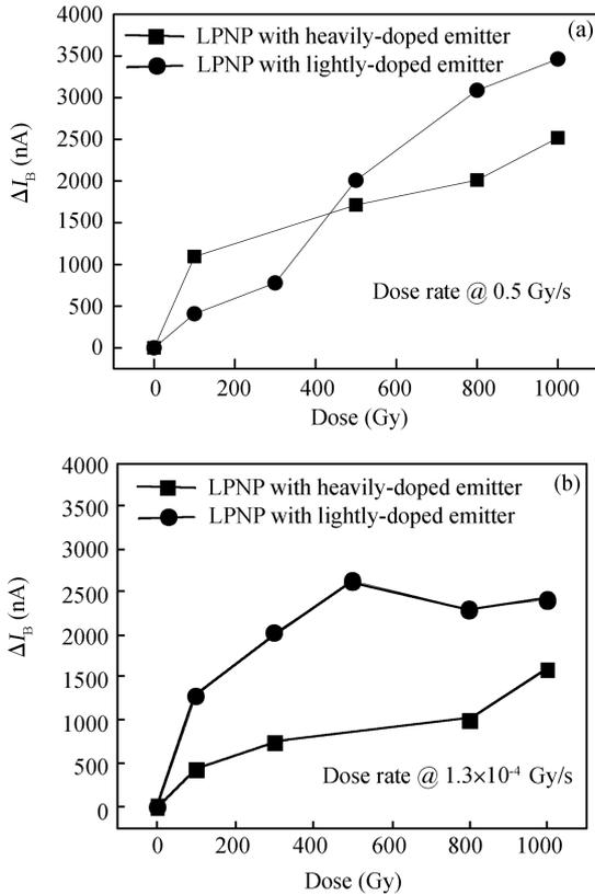
Fig. 2. Excess base current under (a) high- and (b) low-dose-rate irradiation for LPNP transistor with heavily or lightly doped emitters.
