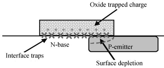
Fig. 4. Positive oxide trapped charge and interface traps near the Si-SiO<sub>2</sub> interface, and the expansion of depletion layer.
