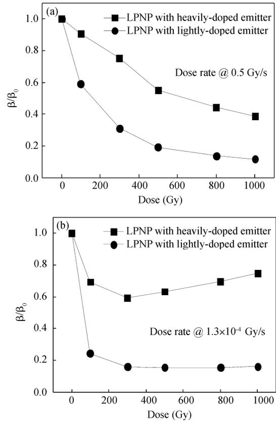
Fig. 3. Normalized current gain of heavily or lightly doped LPNP transistor under (a) high- and (b) low-dose-rate irradiation.
