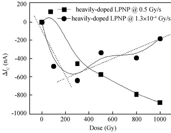
Fig. 5. Collector current of LPNP with heavily doped emitter versus total dose under high- and low-dose-rate irradiation.
