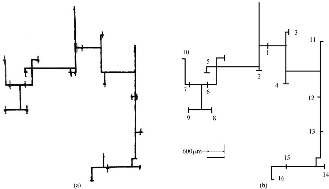
Fig. 5. (a) A clock tree taken from an industrial design. (b) Topology of the clock tree.
