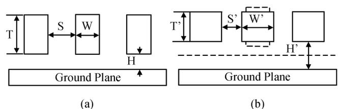
Fig. 1. Cross-section of parallel interconnect lines.
