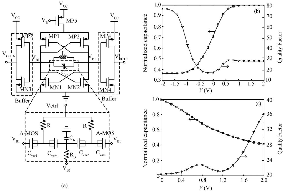
Fig. 3. (a) Schematic of proposed complementary-Gm CMOS LC VCO. (b) Conventional  $C-V$  and  $Q-V$  curve of varactor. (c)  $C-V$  and  $Q-V$  curve of proposed varactor.
