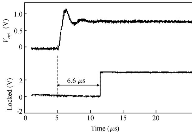
Fig. 9. Measured locking-in time of the proposed PLL.
