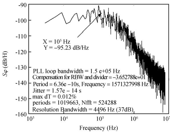
Fig. 5. Simulated phase noise power spectral density of closed-loop PLL.
