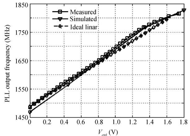
Fig. 7. Simulated and measured PLL tuning curve.
