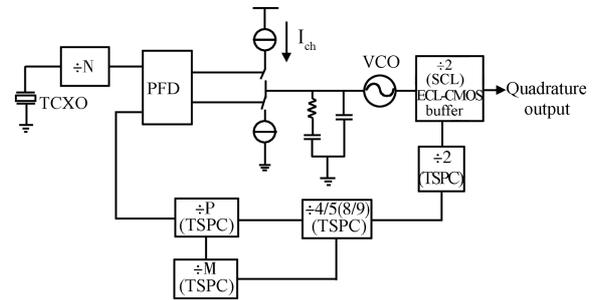
Fig. 2. Block diagram of proposed frequency synthesizer.
