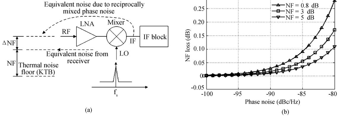
Fig. 1. (a) Reciprocally mixed phase noise and thermal noise floor. (b) Effect of phase noise on NF degradation.
