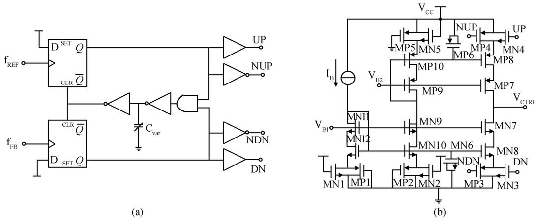
Fig. 4. (a) Simplified schematic of proposed PFD. (b) Schematic of improved charge pump.
