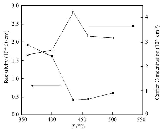
Fig. 1. Carrier concentration and resistance of ITO as a function of temperature.
