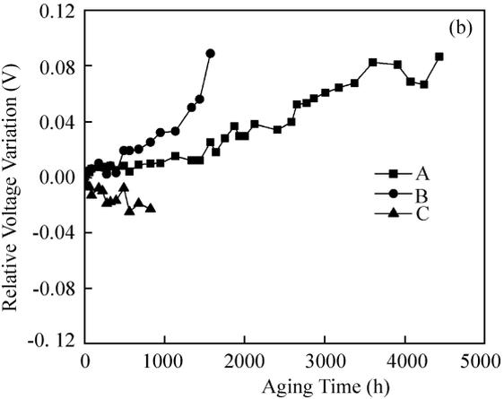
Fig. 7. (a) Output light intensity and (b) voltage variation of the novel LED versus aging time.
