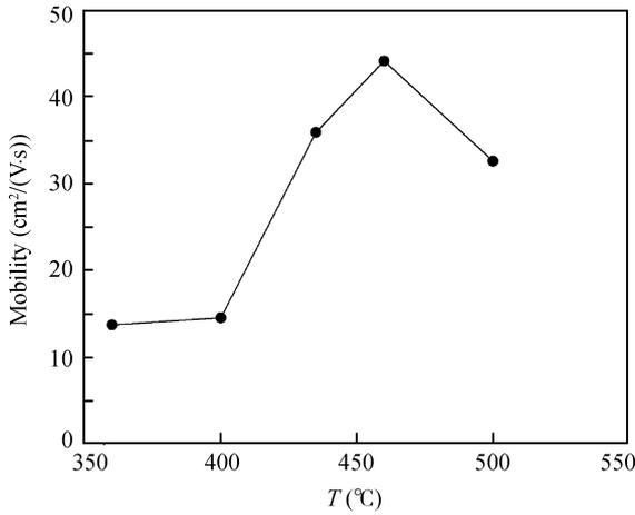
Fig. 2. Mobility of ITO as a function of temperature.
