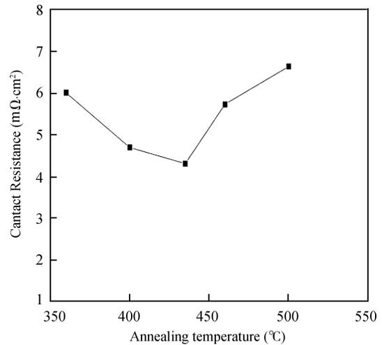
Fig. 4. Specific contact resistance of the ITO/GaP contact as a function of temperature.
