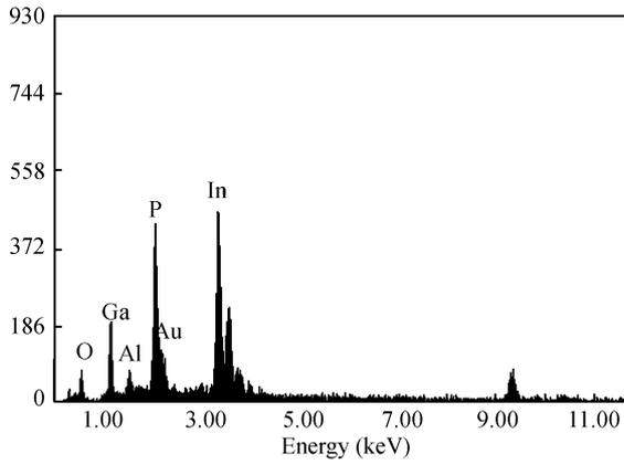
Fig. 5. Auger spectra of the ITO/GaP interface after 435 °C annealing.
