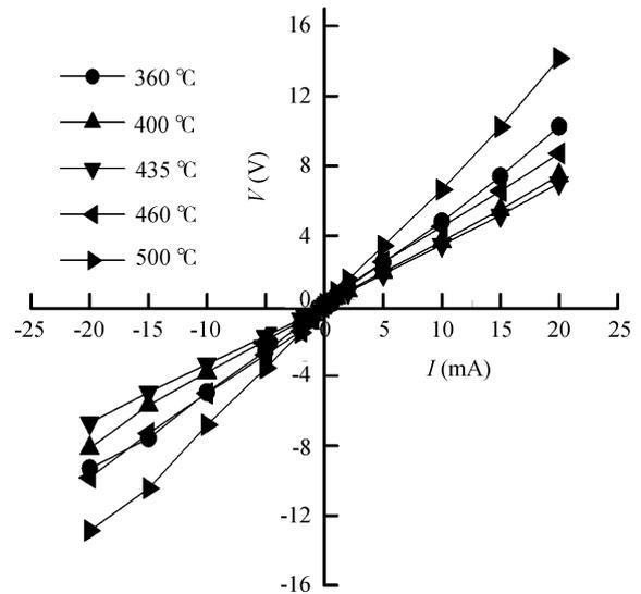
Fig. 3.  $I-V$  characteristics of the ITO /GaP contact as a function of temperature.
