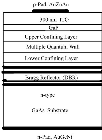
Fig. 6. Structure of AlGaInP LED.
