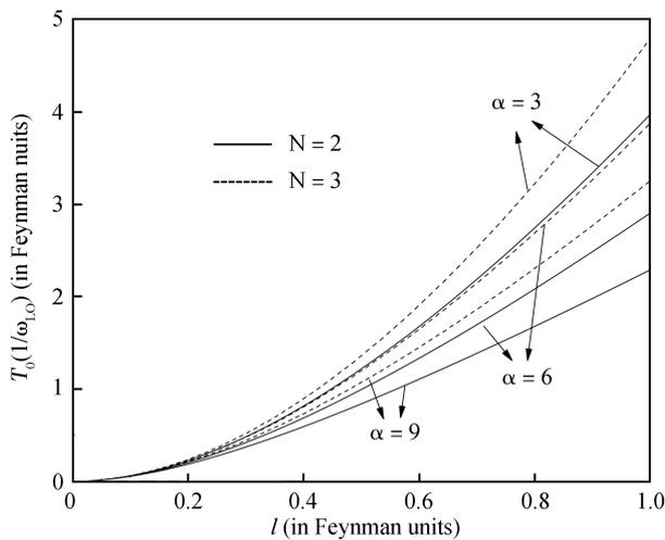
Fig. 3. Period of oscillation as a function of the confinement length  $l$  (in Feynman units) with three coupling strengths. The solid line and the dashed line represent the 2D and 3D, respectively.
