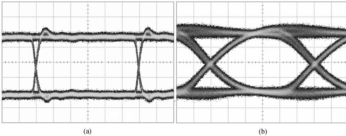
Fig. 8. (a) Optical eye diagrams at 155 Mb/s, 100  $\mu$ W/div, 1.12 ns/div. (b) Optical eye diagrams at 1.25 Gb/s, 100  $\mu$ W/div, 132 ps/div.
