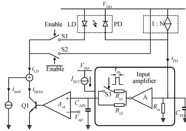
Fig. 2. Block diagram of the proposed fast APC circuit.
