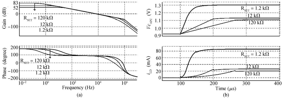
Fig. 4. (a) Frequency response of the open loop. (b) Transient response of the closed loop.
