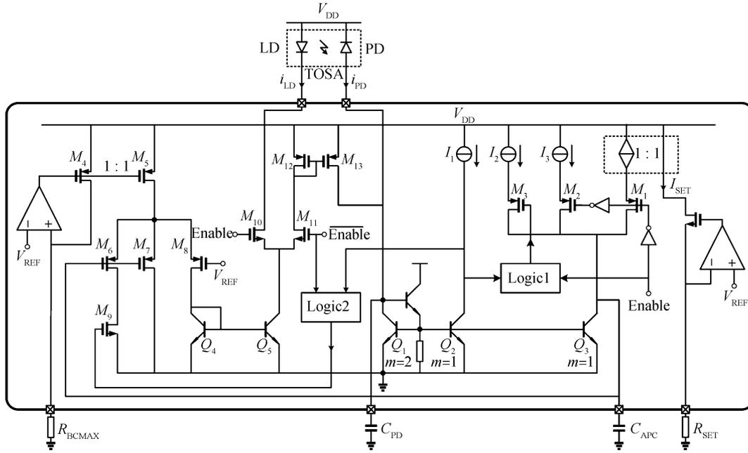
Fig. 3. Simplified schematic of the fast APC circuit.
