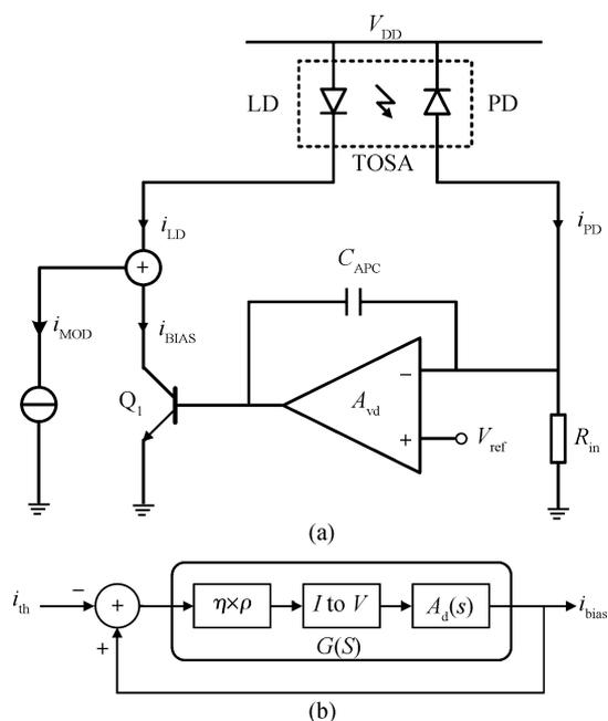
Fig. 1. (a) Block diagram of a traditional APC circuit. (b) Model of (a).
