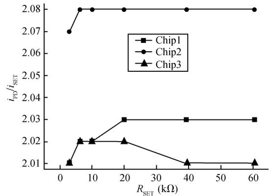
Fig. 6. Setting ratio of  $i_{PD}/i_{SET}$ .
