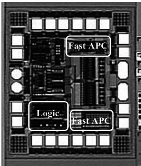
Fig. 5. Die photograph of the LDD with a fast APC.
