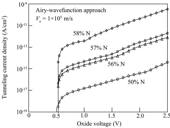
Fig. 4. Electron tunneling current density in the MOS capacitor for several nitrogen compositions of  $TiN_x$  calculated using the Airy-wavefunction approach.
