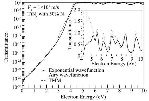
Fig. 2. Electron energy dependence of transmittance of an electron in valley 1 (V1) in which the gate electron phase velocity is  $1 \times 10^5$  m/s.
