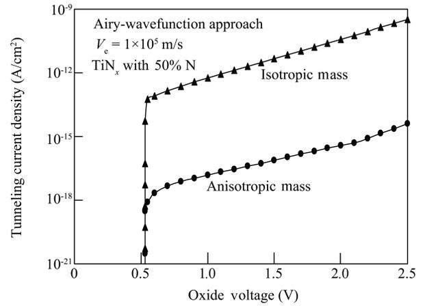
Fig. 5. Tunneling currents calculated by employing the Airy-wavefunction approach under the isotropic and anisotropic masses.
