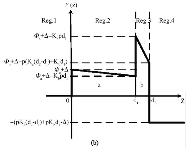
Fig. 1. (a) Energy band diagram of a TiN<sub>x</sub>/HfO<sub>2</sub>/SiO<sub>2</sub>/p-Si MOS capacitor in a flatband condition. (b) Potential profile in the  $z$ -direction under a negative bias voltage applied to the TiN<sub>x</sub> gate.
