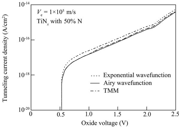
Fig. 3. Tunneling current as a function of oxide voltage for the gate electron phase velocity of  $1 \times 10^5$  m/s.
