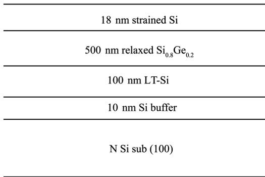
Fig. 1. Structure of the epitaxy layers for biaxial strained-Si material based on LT-Si technology.
