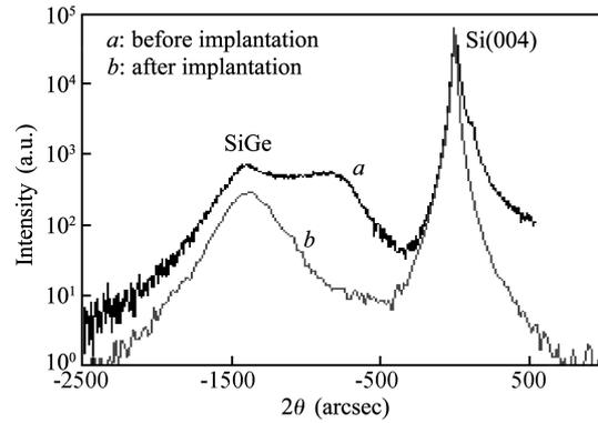
Fig. 3. DCXRD rocking curves of the sample before (curve *a*) and after (curve *b*) P<sup>+</sup> implantation and RTA.
