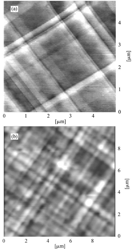
Fig. 5. AFM testing photos of the sample. (a) Before  $\text{P}^+$  implantation and RTA. (b) After  $\text{P}^+$  implantation and RTA.
