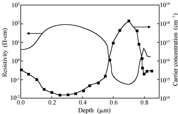
Fig. 2. P<sup>+</sup> distribution within the sample after ion implantation and RTA.
