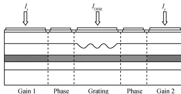
Fig. 1. Schematic diagram of the DBR self-pulsation laser.
