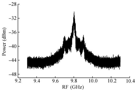
Fig. 3. Typical RF spectrum of the device.  $I_f$ ,  $I_r$  and  $I_{DBR}$  are 108.3 mA, 106 mA and 9 mA respectively and the 3-dB linewidth is about 10 MHz. Measured by RB = 300 kHz, VB = 10 kHz.
