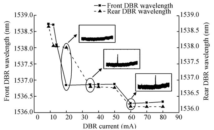
Fig. 5. Wavelength tuned by the increase of  $I_{DBR}$ .
