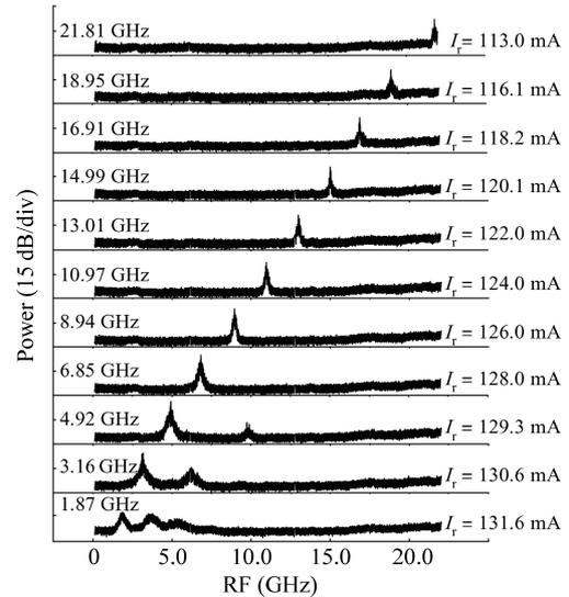
Fig. 4. RF spectra of the device.  $I_f$  and  $I_{DBR}$  are fixed at 108.3 mA, 9 mA with  $I_r$  varied as denoted. Measured by RB = 3 MHz, VB = 300 kHz.
