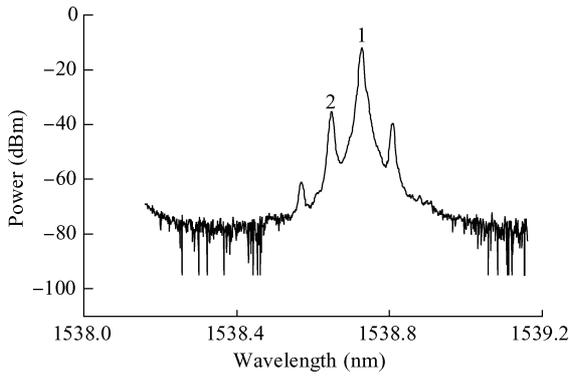
Fig. 2. Typical optical spectrum of the device.  $I_f$ ,  $I_r$  and  $I_{DBR}$  are 108.3 mA, 106 mA and 9 mA respectively.
