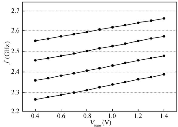
Fig. 10. Measured tuning characteristic of the VCO.
