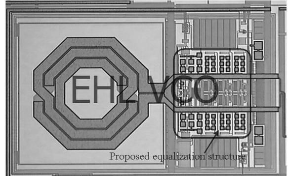
Fig. 9. Micrograph of proposed VCO.
