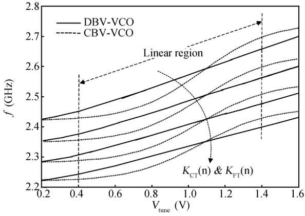
Fig. 4. Simulated  $f-V$  characteristic of different VCO structures.
