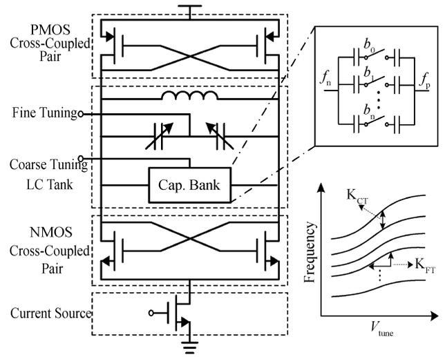
Fig. 2. Schematic and tuning characteristic of conventional CMOS LC-VCO.
