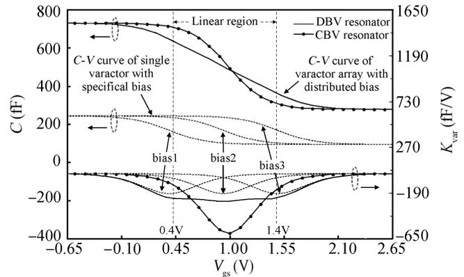
Fig. 3. Simulated  $C-V$  characteristic and  $K_{var}$ .
