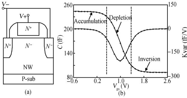
Fig. 1. AMOS varactor. (a) Structure and operation. (b)  $C-V$  characteristic.
