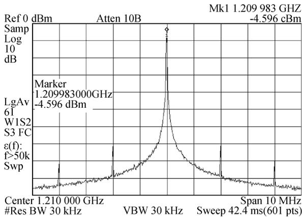
Fig. 11. Measured LO output spectrum.
