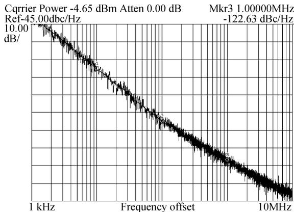
Fig. 12. Measured LO output phase noise at 1-MHz offset.
