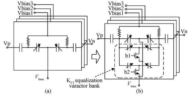
Fig. 5. Conventional DBV resonator. (b) Proposed equalization structure base on switched-varactor DBV resonator.
