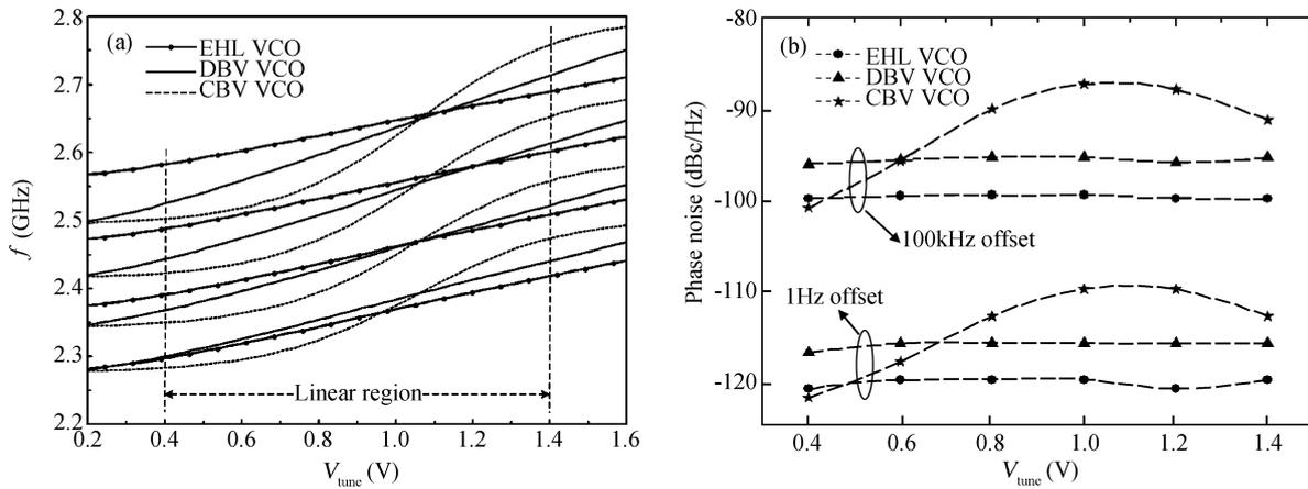
Fig. 7. Simulated results of different VCO structures. (a)  $f-V$  characteristic. (b) Phase noise.
