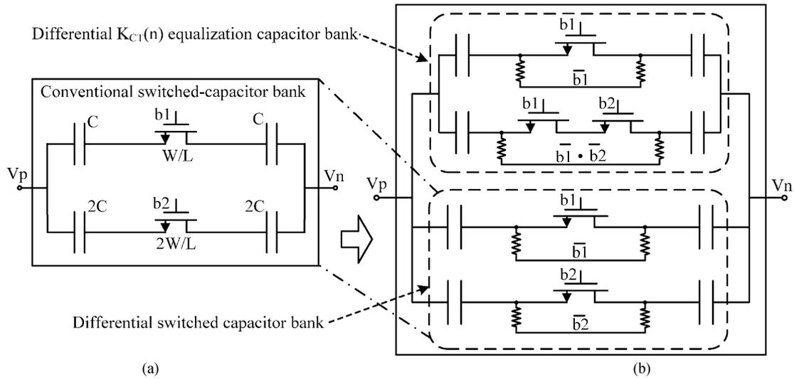
Fig. 6. (a) Conventional binary-weighted structure. (b) Proposed equalization structure base on differential switched-capacitor.
