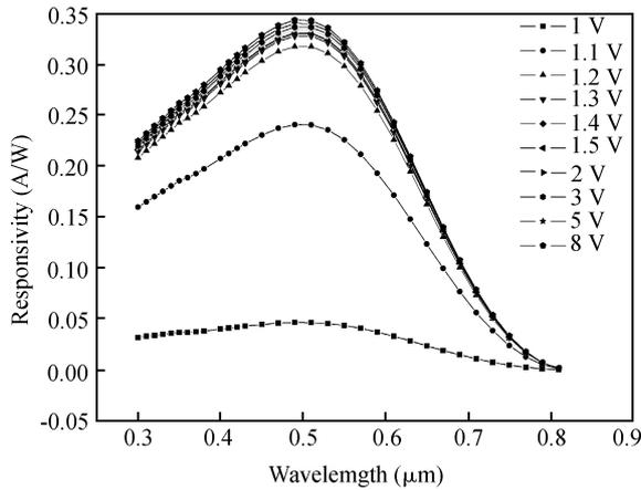
Fig. 6. Response spectra at different biased voltages.
