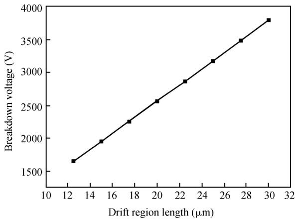
Fig. 3. Linear relationships with drift region and breakdown voltage.
