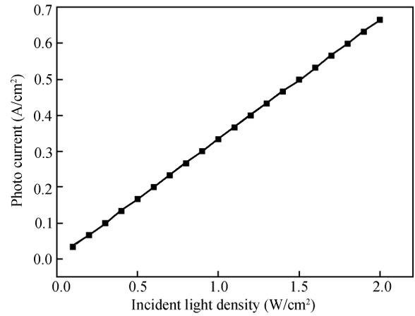
Fig. 4. Photocurrent versus incident light intensity.
