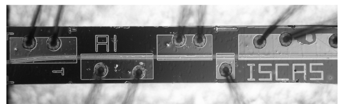
Fig. 1. SGDBR laser with integrated SOA, side-view schematic and micrograph.
