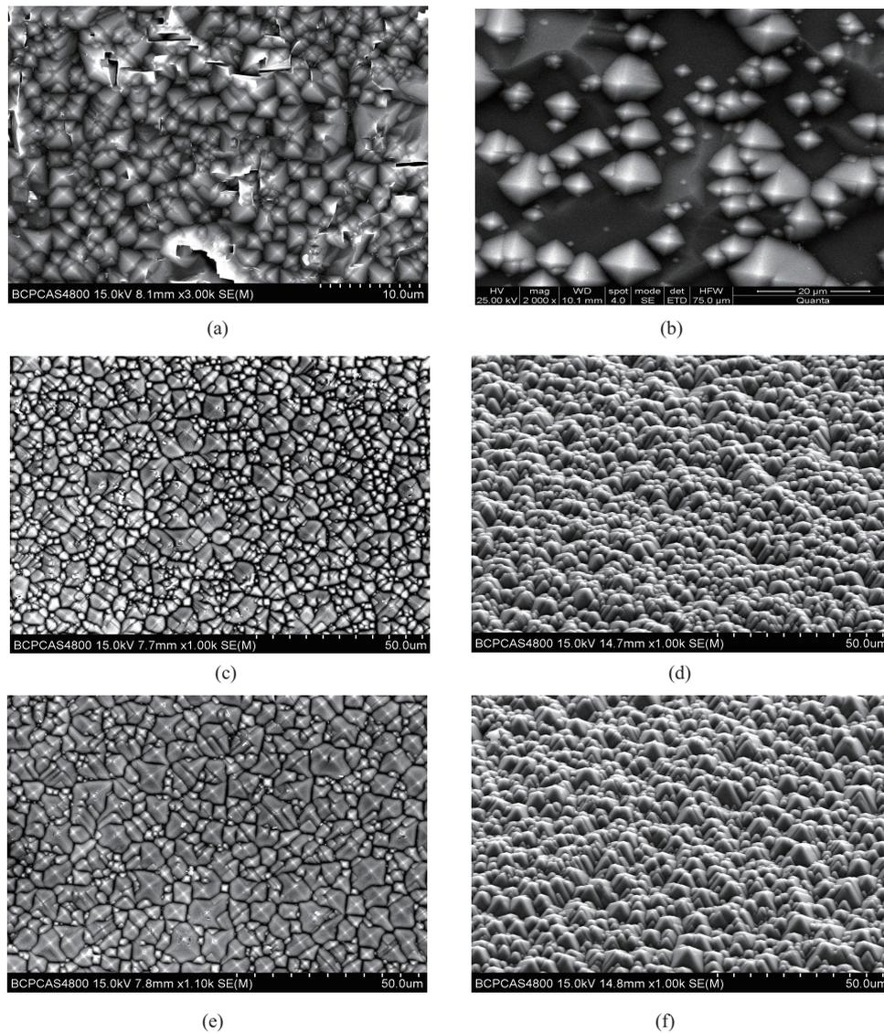
Fig. 2. SEM pictures of the resulting surface morphology in different TMAH concentrations at a temperature of 80 °C. (a) 20 vol.% TMAH for 30 min. (b) 60 vol.% TMAH for 15 min. (c), (d) 30 vol.% TMAH for 30 min. (e), (f) 40 vol.% TMAH for 30 min.
