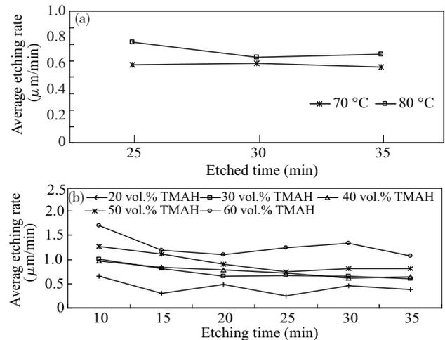
Fig. 1. Average etching rates versus etching time. (a) 40 vol.% TMAH at temperatures of 70 °C and 80 °C. (b) Different TMAH concentrations at a temperature of 80 °C.
