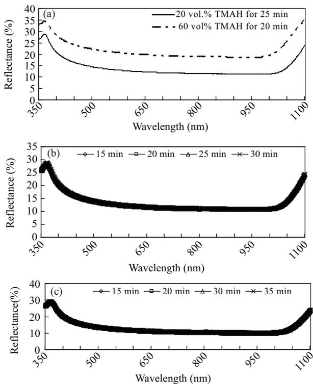
Fig. 3. Textured surface reflectance versus wavelength at  $80^\circ$  for different etching times. (a) 20 vol.% TMAH and 60 vol.% TMAH. (b) 30 vol.% TMAH. (c) 40 vol.% TMAH.
