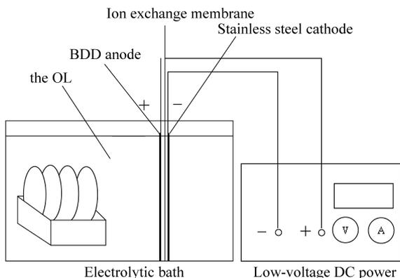
Fig. 2. Setup of the BDD film anode electrochemical oxidation.
