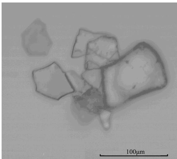
Fig. 3. Sheet micelles observed with 500 times magnification.
