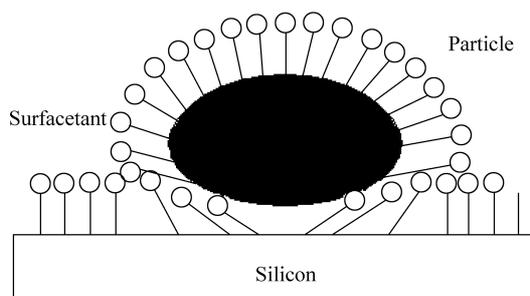
Fig. 1. Non-ionic surfactant film adsorption on the silicon surface and around a particle.
