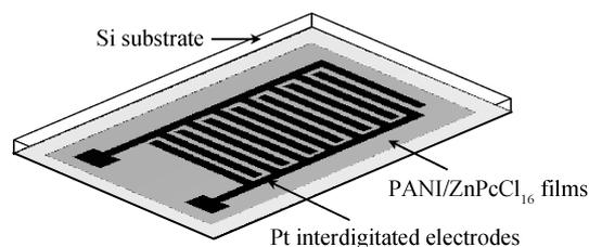
Fig. 1. Schematic diagram of interdigitated electrodes for PANI/ZnPcCl<sub>16</sub> sensors.
