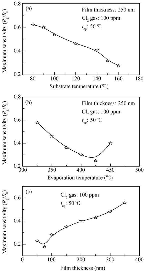
Fig. 2. Maximum sensitivity of PANI/ZnPcCl<sub>16</sub> sensors influenced by the coevaporation condition. (a) Substrate temperature. (b) Evaporation temperature. (c) Film thickness.
