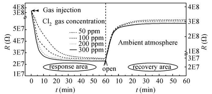
Fig. 4. Response and recovery of PANI/ZnPcCl<sub>16</sub> sensors operated at 100 °C (film thickness: 75 nm).
