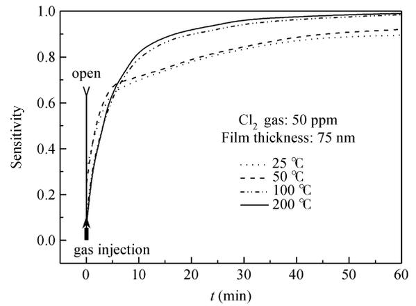
Fig. 3. Transient response of PANI/ZnPcCl<sub>16</sub> sensors operated at different temperatures.
