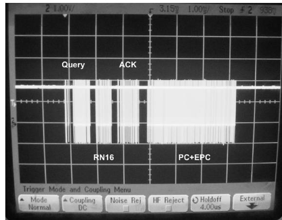
Fig. 12. Communication procedure between the proposed reader and tags.
