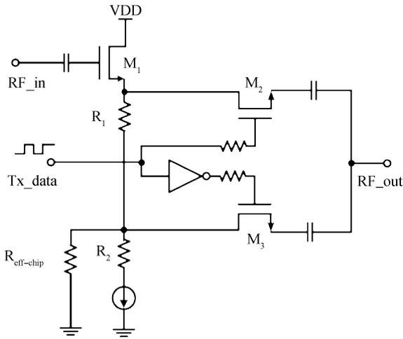
Fig. 5. Schematic of the modulator.
