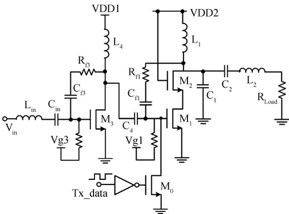
Fig. 6. Schematic of the class-E PA.
