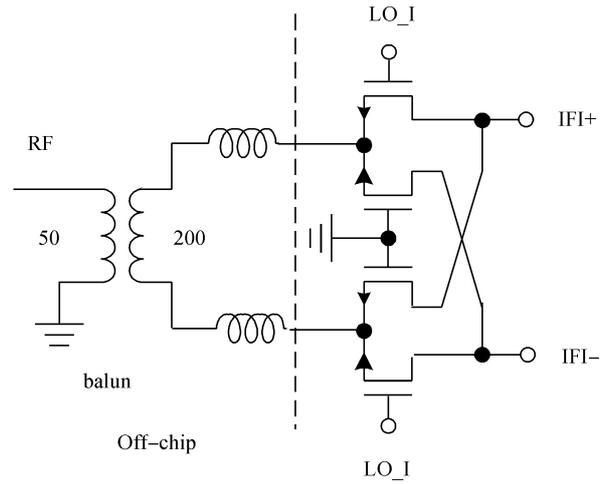
Fig. 7. Schematic of the down-conversion mixer.
