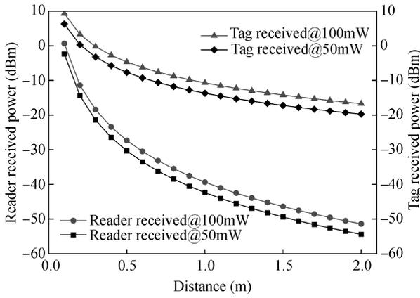
Fig. 2. Power received by the tag and power received by the reader versus distance between the reader and tag.
