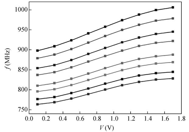
Fig. 11. Measured VCO tuning curve after divider.
