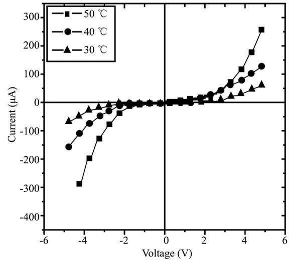
Fig. 3. Current–voltage characteristics of the n-Si/CuPc hetero-junction at 30, 40, and 50 °C.
