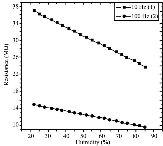
Fig. 6. Change in device resistance as a function of humidity.
