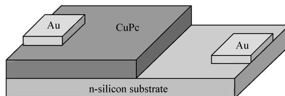
Fig. 1. Schematic view of n-Si/CuPc hetero-junction.
