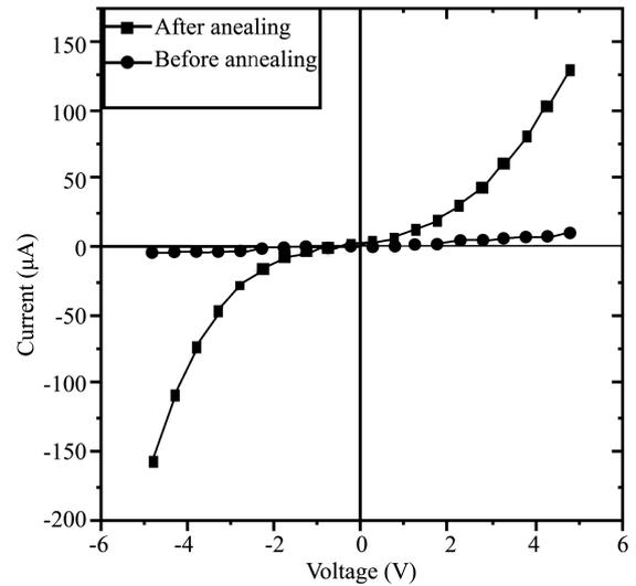
Fig. 2. Current–voltage characteristics of n-Si/CuPc hetero-junction before and after annealing.
