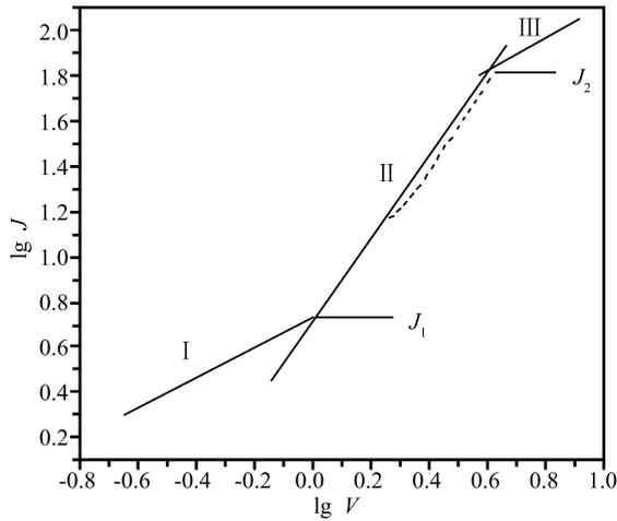
Fig. 4.  $\lg J$  versus  $\lg V$  plot of the n-Si/CuPc hetero-junction in forward bias at room temperature.
