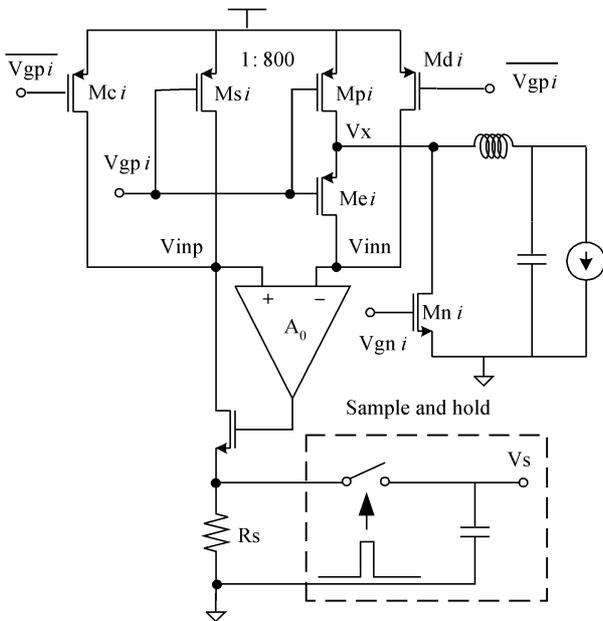
Fig. 2. An improved current sensing circuit for the width controller.
