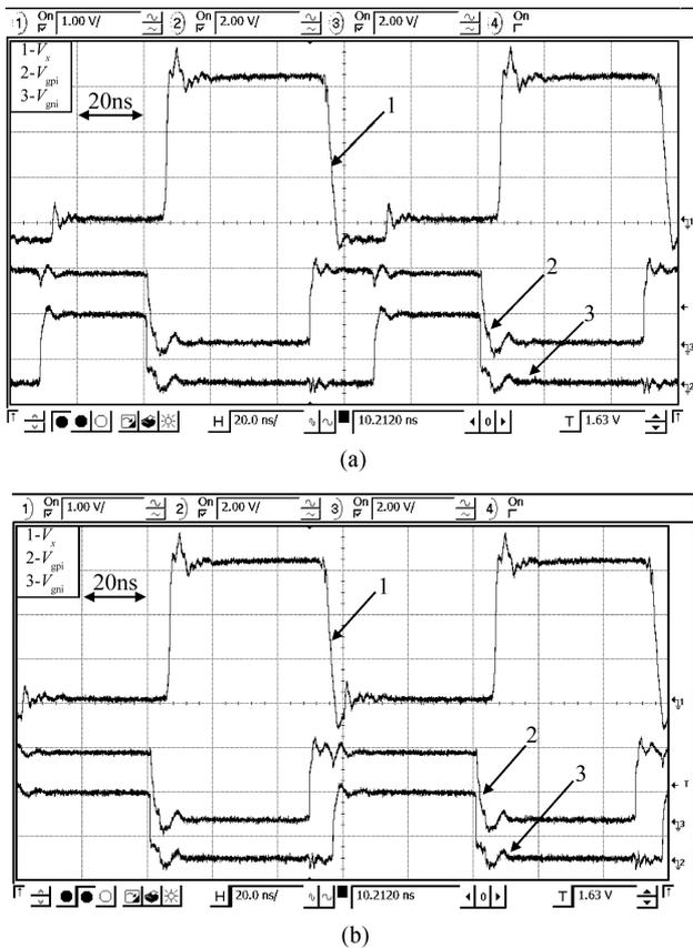
Fig. 7. Waveforms of  $V_x$ ,  $V_{gpi}$  and  $V_{gmi}$  (a) without optimal dead time adjustment and (b) with optimal dead time adjustment.
