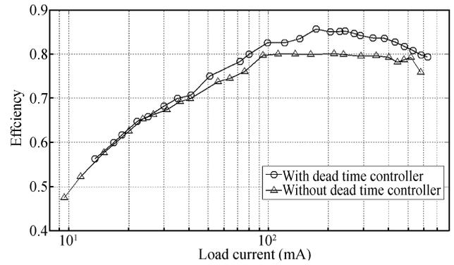
Fig. 8. Efficiency comparison with and without dead time controller.
