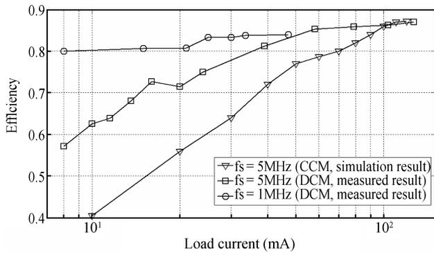
Fig. 10. Efficiency comparison between DCM and CCM ( $V_{\text{in}} = 3.6 \text{ V}$ ,  $V_{\text{out}} = 1.8 \text{ V}$ ).
