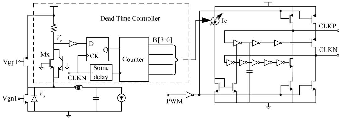
Fig. 4. A novel optimal dead time controller.
