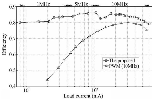
Fig. 11. Measured efficiency with and without proposed techniques ( $V_{\text{in}} = 3.6 \text{ V}$ ,  $V_{\text{out}} = 1.8 \text{ V}$ ).
