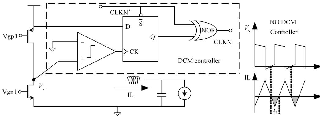
Fig. 5. DCM controller circuit and the waveform of  $V_x$  and  $I_L$  without the DCM controller.
