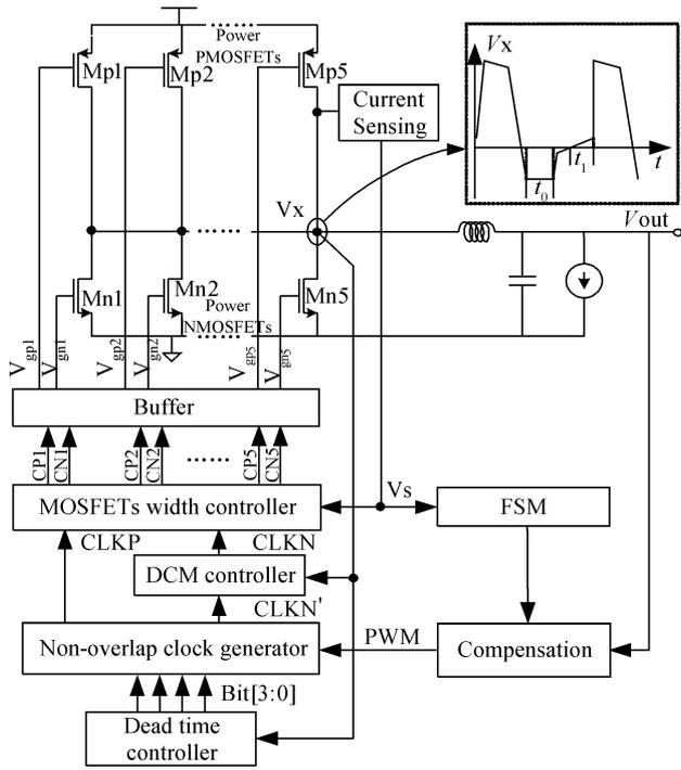
Fig. 1. Architecture of the proposed controllers for the buck DC-DC converter.
