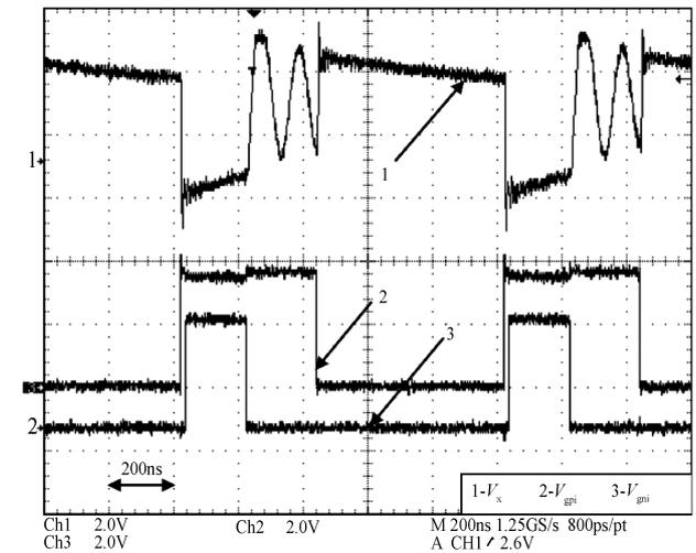
Fig. 9. Waveforms of  $V_x$ ,  $V_{gpi}$  and  $V_{gmi}$  at DCM mode.
