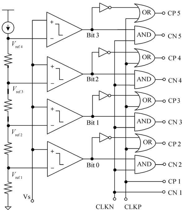
Fig. 3. Width controller for the power PMOSFET and NMOSFET.
