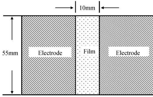
Fig. 1. Schematic diagram of a PbI<sub>2</sub> film with Al electrodes.
