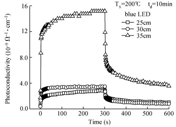
Fig. 3. Dependence of PbI<sub>2</sub> film's photoconductivity on source–substrate distance.
