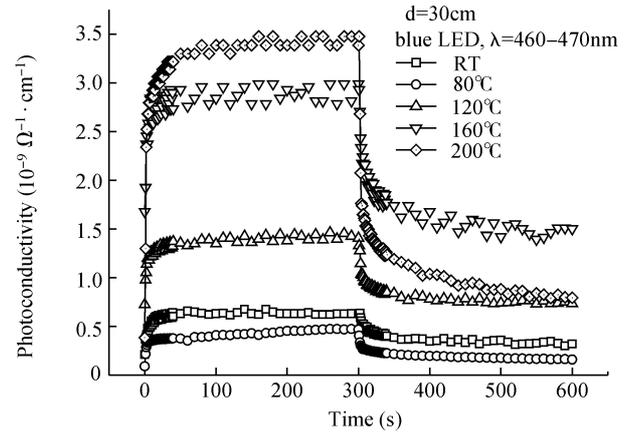
Fig. 2. Dependence of PbI<sub>2</sub> film's photoconductivity on substrate temperature.
