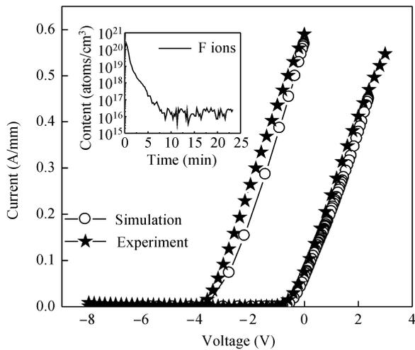
Fig. 4. Comparisons of the simulation and experiment results before and after fluorine plasma treatment of AlGaIn/GaN HEMTs. The inset is the SIMS result for the sample treated by fluorine plasma.
