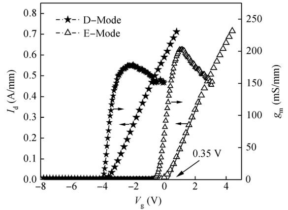
Fig. 2. Transfer and transconductance characteristics of the depletion-mode and enhancement-mode AlGaIn/GaN HEMTs.
