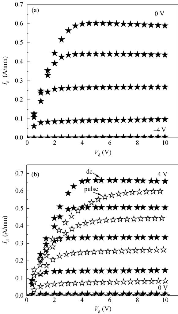
Fig. 1. (a) DC  $I-V$  characteristic of a depletion-mode AlGaIn/GaN HEMT. (b) DC and pulsed  $I-V$  characteristic of an enhancement-mode AlGaIn/GaN HEMT.
