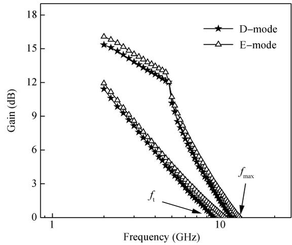
Fig. 3. Small-signal characteristics of the depletion-mode and enhancement-mode AlGaIn/GaN HEMTs.
