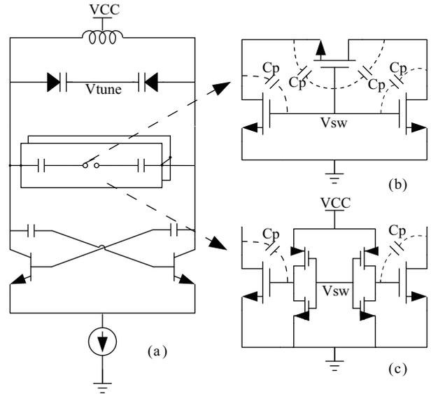
Fig. 3. (a) VCO architecture. (b) Conventional switch with large parallel parasitic capacitance  $C_p$ . (c) Proposed switch with small size inverters to isolate parasitic coupling.
