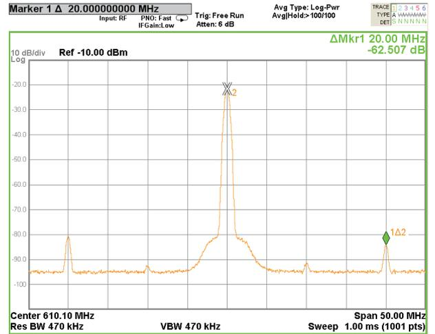
Fig. 11. U-band spectrum and reference spur for fractional-*N* mode.
