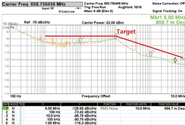
Fig. 10. S-band phase noise @ 658.75 MHz (after divide-by-4).
