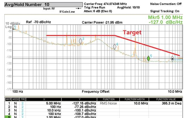
Fig. 8. U-band integer-*N* phase noise @ 474 MHz.
