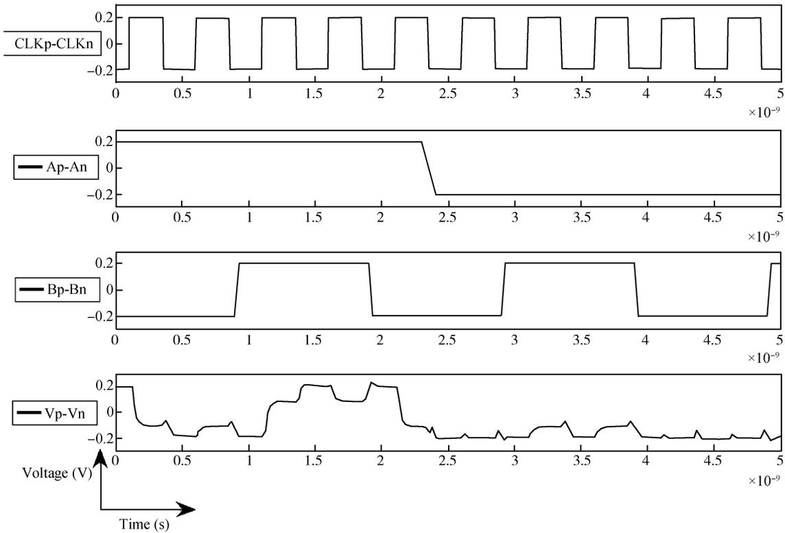
Fig. 6. Timing diagram of the proposed D-latch.
