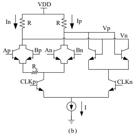
Fig. 5. (a) Conventional-latch with AND function. (b) Proposed D-latch with AND function.
