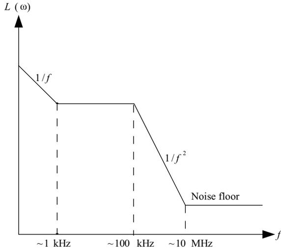
Fig. 2. Phase noise spectrum in locked PLL.
