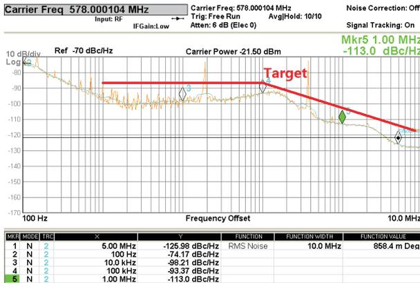
Fig. 9. U-band fractional-*N* phase noise @ 578 MHz.
