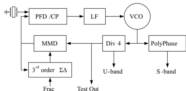
Fig. 1. Block diagram of the PLL.
