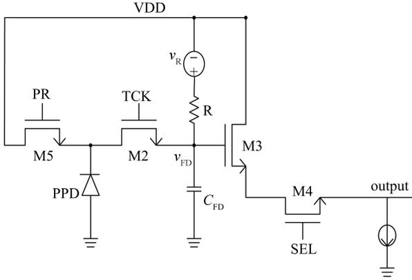
Fig. 3. Equivalent circuit of five-transistor pixel.
