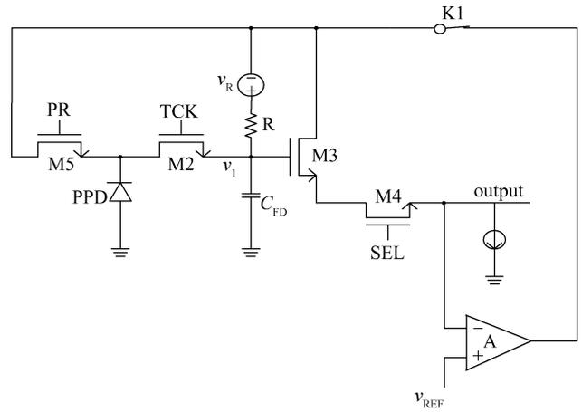
Fig. 5. Equivalent circuit of proposed feedback reset.
