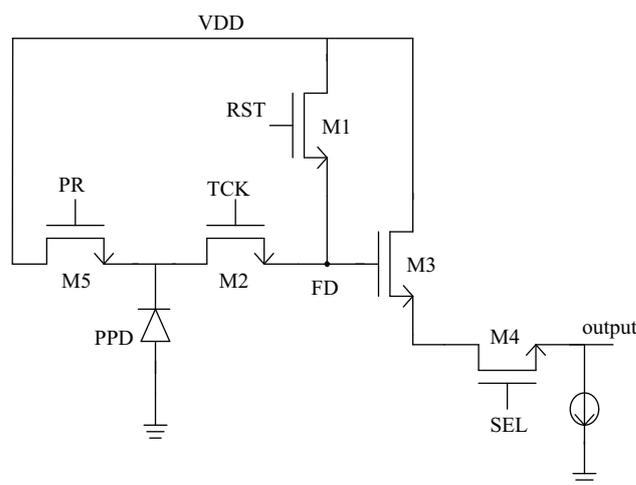
Fig. 1. Pixel structure diagram.
