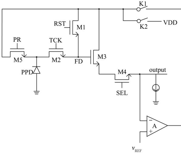
Fig. 4. Proposed feedback reset schematic.
