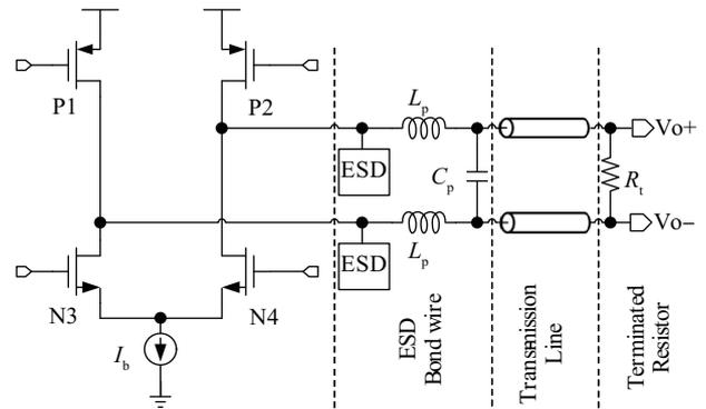
Fig. 7. Simulation circuit of LVDS driver.
