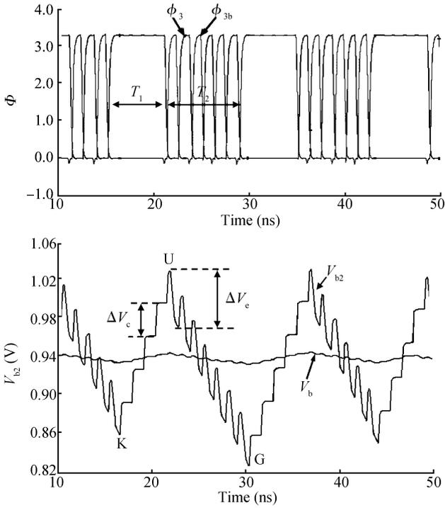
Fig. 5.  $V_{b2}$  changed as node A charge/discharge.
