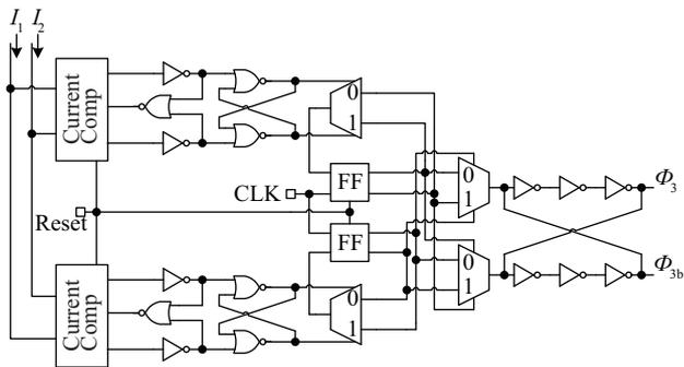
Fig. 3. Control logic of charge/discharge capacitors.
