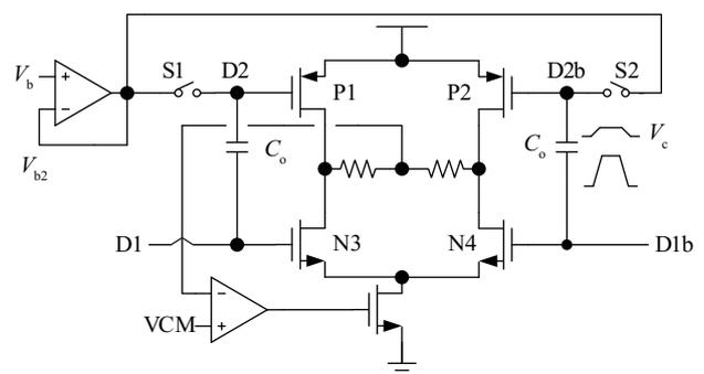
Fig. 1. Single current source LVDS driver.
