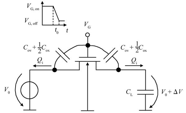
Fig. 4. Charge injection model of a MOS transistor.
