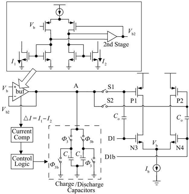
Fig. 2. Modified LVDS driver upon Fig. 3 (CMFB not shown).
