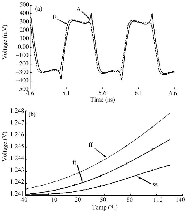
Fig. 8. Simulated output differential and common-mode signal of proposed LVDS driver. (a) Output differential voltage. (b) Output common-mode voltage.
