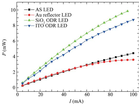
Fig. 2. Characteristic of four samples between current and optical output power.
