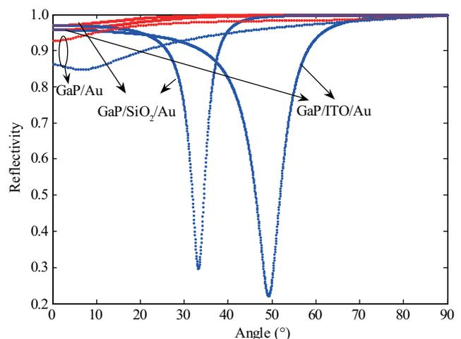
Fig. 1. Calculated reflectivity versus angle of incidence for an Au reflector, a SiO<sub>2</sub> ODR and an ITO ODR.
