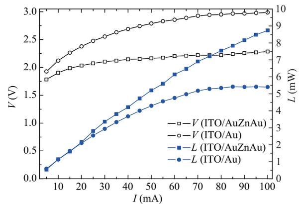
Fig. 3.  $I$ - $V$  and  $L$ - $I$  curves of ITO ODR LEDs with and without Zn.
