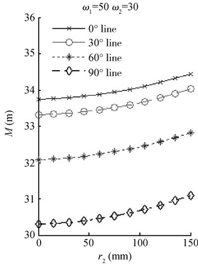
Fig. 2. Relationship between  $M$  and  $r_2$  at inclination angles of  $0^\circ$ ,  $30^\circ$ ,  $60^\circ$ ,  $90^\circ$  ( $\mu = 400$  mm/min,  $L = 50$  mm).
