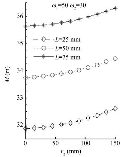
Fig. 3. Relationship between  $M$  and  $r_2$  in reciprocating scope of 25 mm, 50 mm, 75 mm ( $\mu = 400$  mm/min,  $\theta = 0^\circ$ ).
