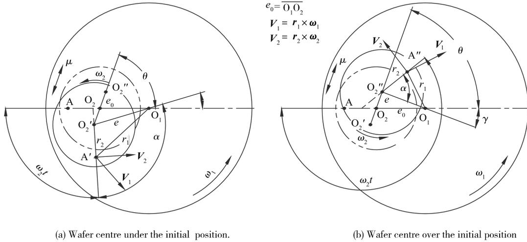
Fig. 1. Kinematic relations of line-orbit CMP in the situations (a) and (b).
