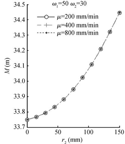
Fig. 4. Material removal rate at the reciprocating speed of 200, 400 and 800 mm/min ( $L = 50$  mm,  $\theta = 0^\circ$ ).
