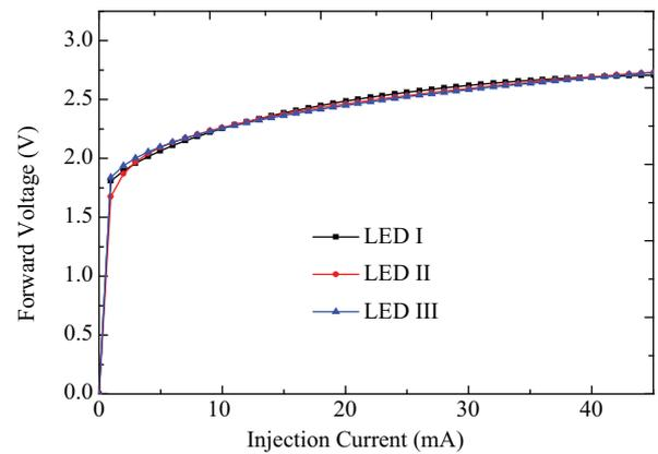
Fig. 2. Typical *I*-*V* characteristics of LED I, LED II and LED III.
