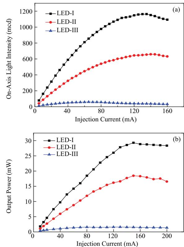
Fig. 3. (a) Relationship between the pulse current injection and on-axis light intensity of LEDs I, II and III. (b) Relationship between the direct current injection and the light output power of LEDs I, II and III.
