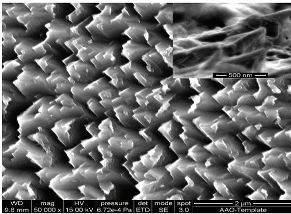
Fig. 4. Scanning electron micrograph (SEM) image of the roughened surface of the LED after the wet etching
