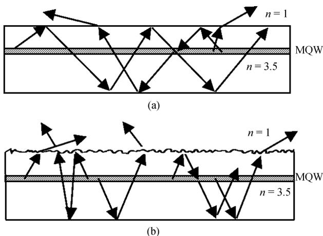
Fig. 5. Possible photons paths inside the structures of (a) LED-II and (b) LED-I.
