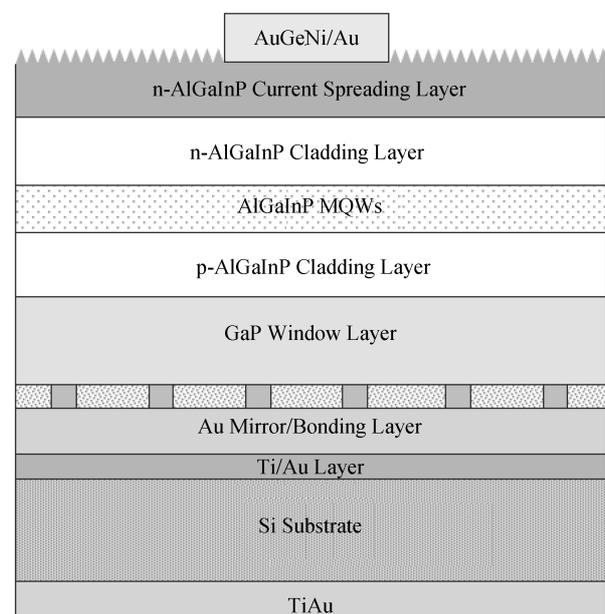
Fig. 1. Schematic cross section of an LED with metal bonding and surface roughening.
