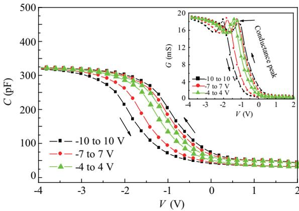
Fig. 5.  $C-V$  and  $G-V$  (inset) characteristics of memory devices with medium density Au nanocrystal monolayer.
