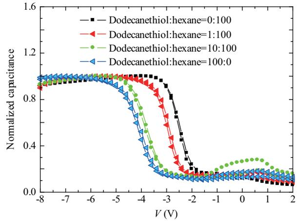
Fig. 7.  $C-V$  curve shift toward negative bias with increasing density of dodecanethiol molecules within the sandwich memory structure of four reference samples.
