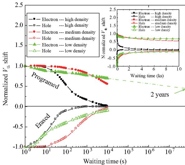
Fig. 8. Data retention of memory devices with Au nanocrystal monolayer of three different densities with a logarithmic and linear (inset) scale of horizontal axis.
