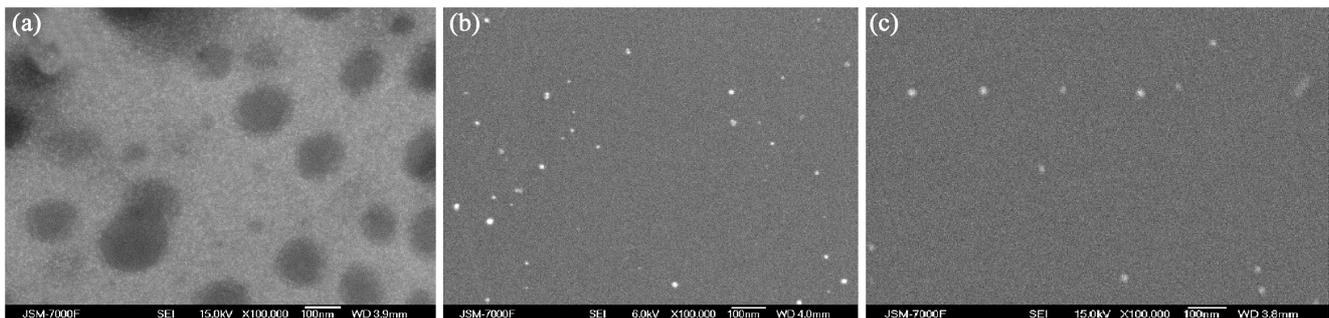
Fig. 3. SEM images of Au nanocrystal monolayer with (a) high density, (b) medium density and (c) low density.
