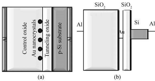
Fig. 1. (a) Schematic illustration and (b) energy band diagram of metal nanocrystal nonvolatile memory devices.
