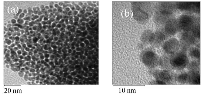
Fig. 2. (a) TEM and (b) HRTEM image of colloid Au nanocrystals.
