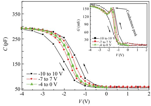
Fig. 6.  $C-V$  and  $G-V$  (inset) characteristics of memory devices with low density Au nanocrystal monolayer.
