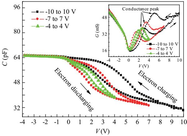
Fig. 4.  $C-V$  and  $G-V$  (inset) characteristics of memory devices with high density Au nanocrystal monolayer.
