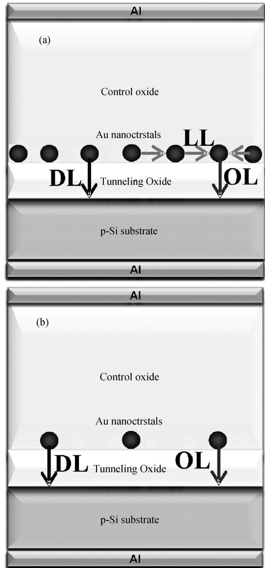
Fig. 9. Illustration of charge loss mechanisms of nonvolatile memory devices with (a) high density nanocrystals monolayer and (b) medium or low density nanocrystals monolayer.
