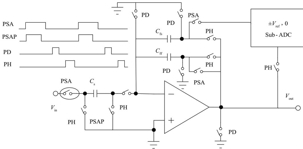
Fig. 3. Schematic of the SMDAC.s
