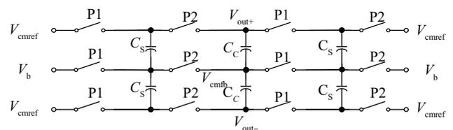
Fig. 7. Common-mode feedback circuit.
