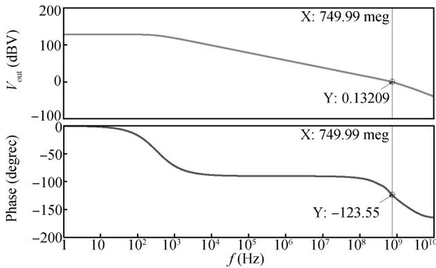
Fig. 6. Simulated frequency response of the amplifier.
