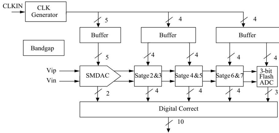
Fig. 1. Proposed ADC architecture.
