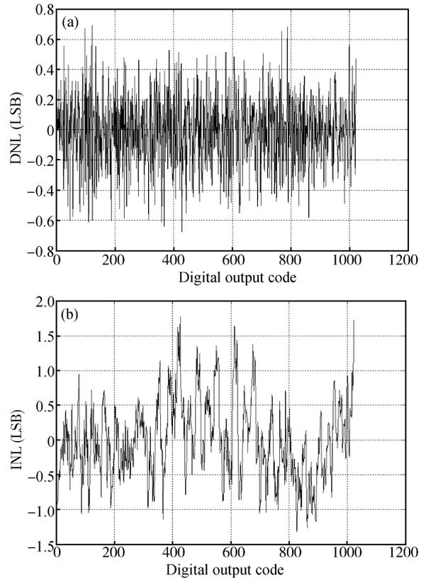
Fig. 11. Measured static performance. (a) DNL. (b) INL.
