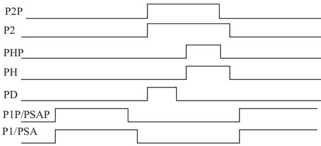
Fig. 2. Timing diagram of the ADC.
