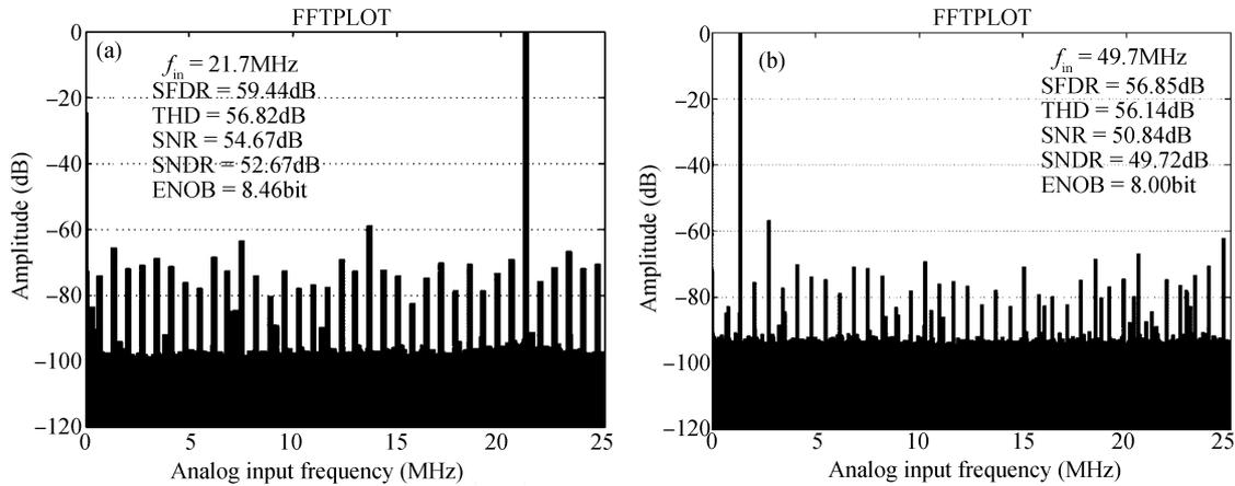
Fig. 12. Measured FFT plots @  $f_s = 50$  MS/s. (a) 21.7-MHz input. (b) 49.7-MHz input.
