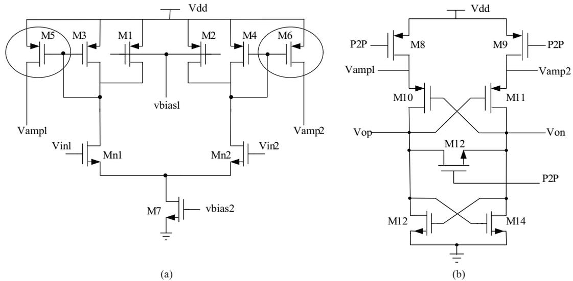
Fig. 9. Comparator. (a) Pre-amplifier. (b) Latch.
