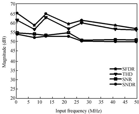
Fig. 13. Measured dynamic performance versus input frequency.
