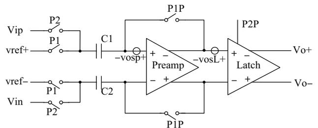
Fig. 8. Schematic of the comparator.
