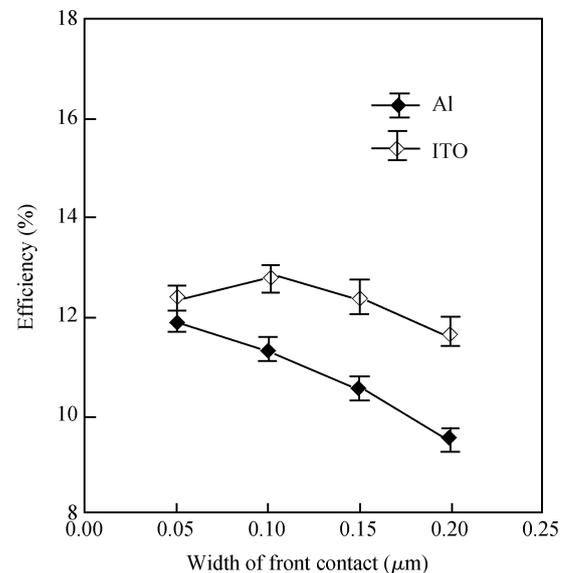
Fig. 5. Dependence of maximum conversion efficiency on the width of the contact electrode for devices with Al and ITO electrodes, respectively, and with a  $p^+$  layer of  $0.1 \mu\text{m}$  thickness and an i-layer of  $20 \mu\text{m}$  thickness.
