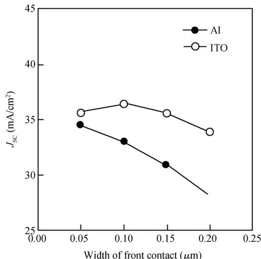
Fig. 2. Dependence of short-circuit current on the width of contact electrode for devices with Al and ITO electrodes, respectively, and with a p<sup>+</sup> layer of 0.1 μm thickness and an i-layer of 20 μm thickness.
