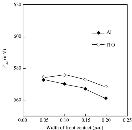
Fig. 4. Dependence of open-circuit voltage on the width of the contact electrode for the devices with Al and ITO electrodes, respectively, and with a  $p^+$  layer of  $0.1 \mu\text{m}$  thickness and an i-layer of  $20 \mu\text{m}$  thickness.
