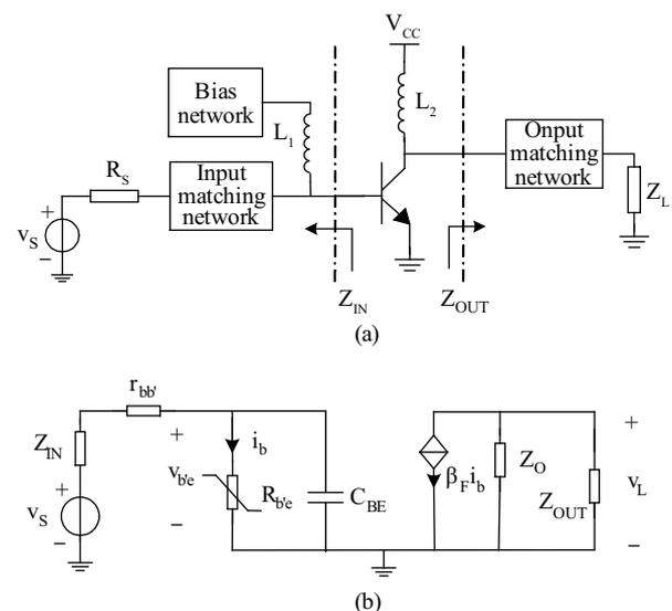
Fig. 1. (a) Typical CE BJT amplifier schematic and (b) its equivalent nonlinear circuit for a Volterra series calculation.
