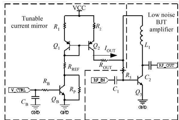
Fig. 6. Schematic of dynamic bias current LNA.
