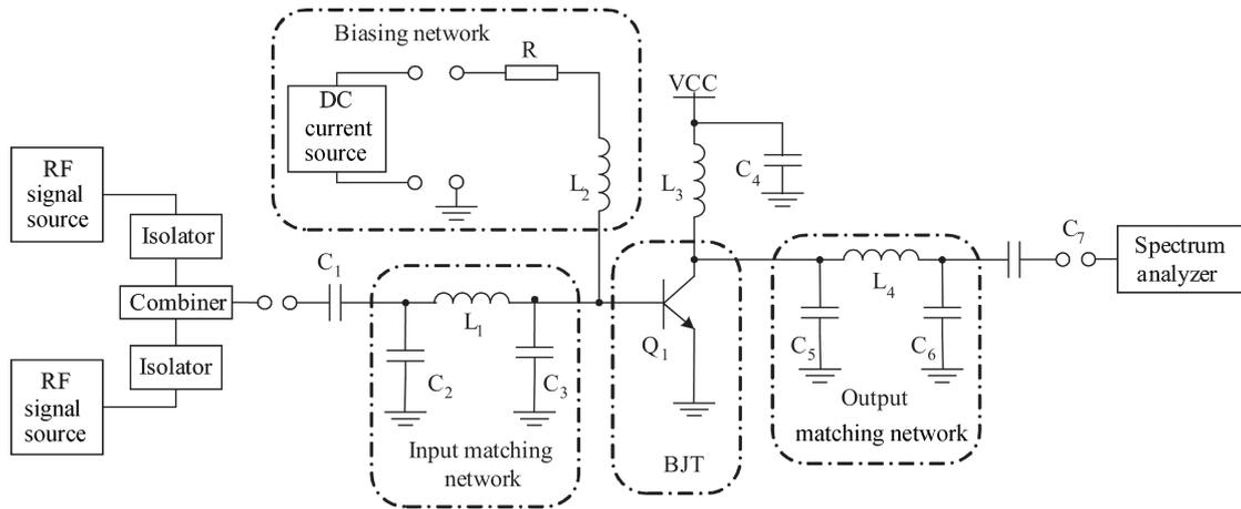
Fig. 4. Circuit used in two-tone test.
