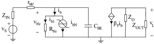
Fig. 2. Linearized circuit for the CE BJT amplifier.
