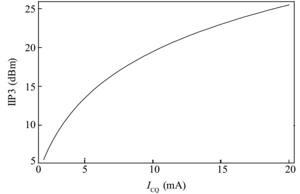
Fig. 3. Calculation curve of IIP3 versus  $I_{CQ}$ .
