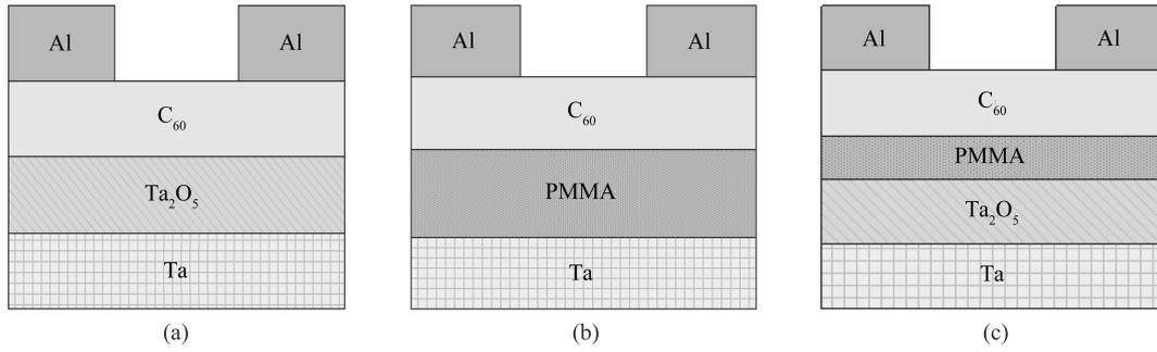
Fig. 1. Schematic cross-sectional structures of OTFTs with (a) Ta<sub>2</sub>O<sub>5</sub> insulator, (b) PMMA insulator, and (c) Ta<sub>2</sub>O<sub>5</sub>/PMMA insulators.
