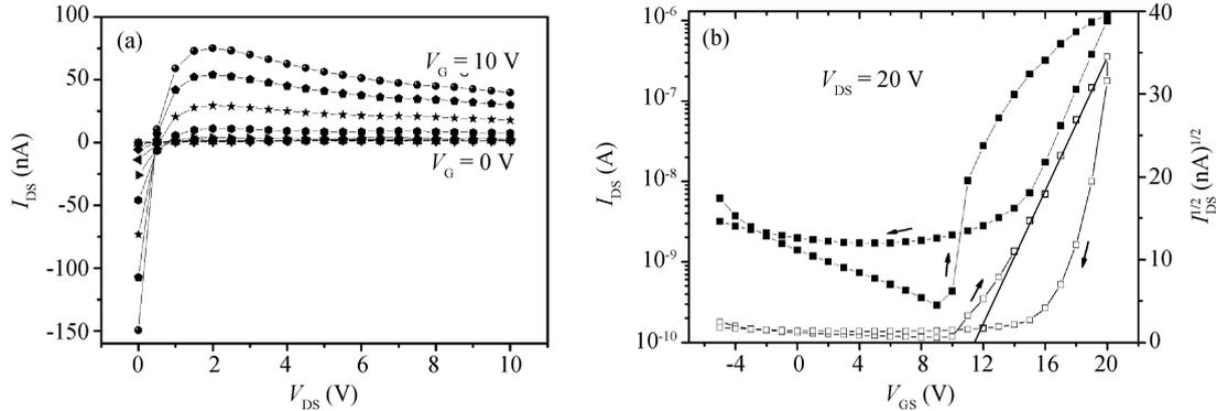
Fig. 2. Electrical characteristics of the OTFT with a Ta<sub>2</sub>O<sub>5</sub> single insulator. (a)  $I_{DS}$  versus  $V_{DS}$  output curve. (b)  $I_{DS}^{1/2}$  and  $\lg I_{DS}$  versus  $V_{GS}$  transfer curve. The voltage is applied in Al electrode.
