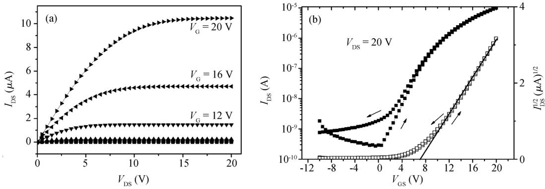
Fig. 3. Electrical characteristics of the OTFT with a PMMA single insulator. (a)  $I_{DS}$  versus  $V_{DS}$  output curve. (b)  $I_{DS}^{1/2}$  and  $\lg I_{DS}$  versus  $V_{GS}$  transfer curve.
