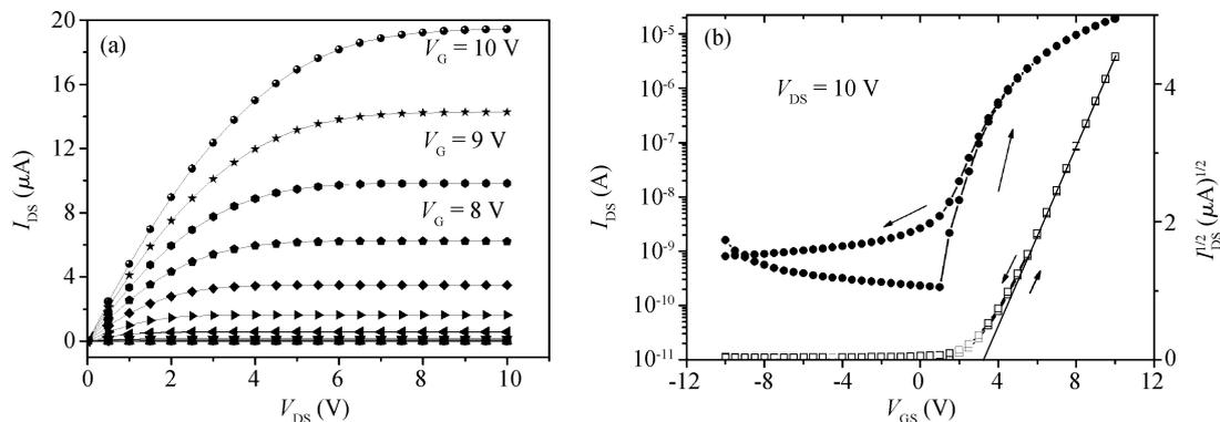
Fig. 5. Electrical characteristics of the OTFT with Ta<sub>2</sub>O<sub>5</sub>/PMMA double insulators. (a)  $I_{DS}$  versus  $V_{DS}$  output curve. (b)  $I_{DS}^{1/2}$  and  $\lg I_{DS}$  versus  $V_{GS}$  transfer curve.
