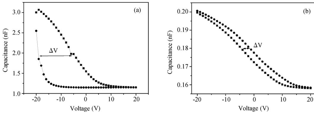
Fig. 4.  $C-V$  characteristic curve of the (a) Ta/Ta<sub>2</sub>O<sub>5</sub>/C<sub>60</sub>/Al and (b) Ta/PMMA/C<sub>60</sub>/Al MIS structures. The voltage is applied in Al electrode.
