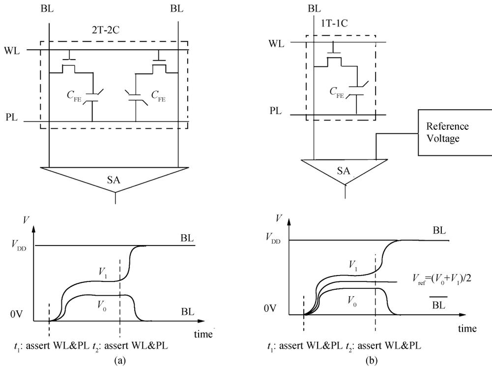
Fig. 1. Reference voltage generation for (a) 2T-2C architecture and (b) 1T-1C architecture<sup>[1]</sup>.
