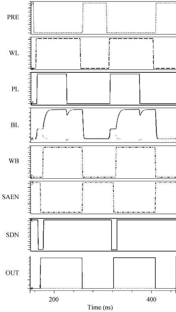
Fig. 4. Timing diagram of the proposed asymmetrical sensing scheme.
