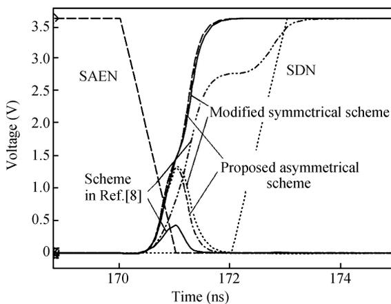
Fig. 6. Comparison of the sensing courses of the schemes mentioned in this paper.
