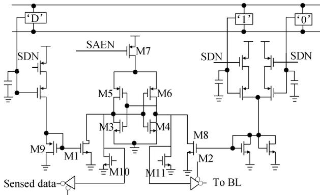
Fig. 2. Conventional symmetrical current-based sensing scheme<sup>[8]</sup>.
