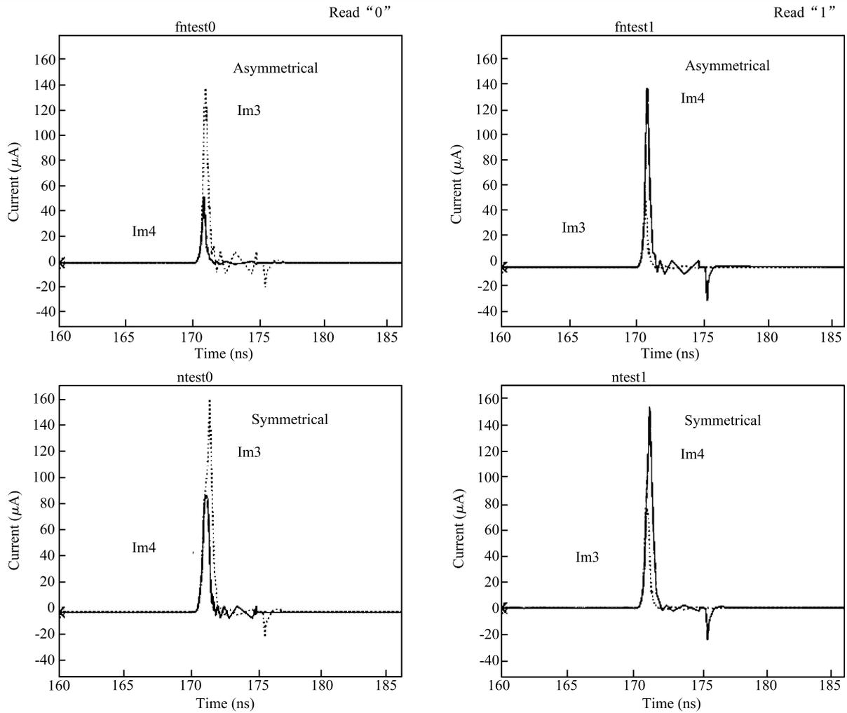
Fig. 5. Sense margins in a read cycle of the proposed asymmetrical scheme and the modified symmetrical scheme.
