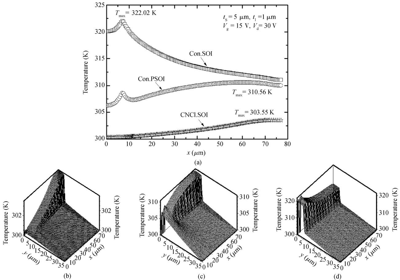
Fig. 5. Thermal characteristics with  $V_d = 30$  V and  $V_g = 15$  V. (a) Surface temperature profiles ( $y = 0.001 \mu\text{m}$ ) for the CNCI PSOI, the conventional PSOI and the SOI. (b) Three-dimensional temperature profiles of the CNCI PSOI. (c) Three-dimensional temperature profiles of the conventional PSOI. (d) Three-dimensional temperature profiles of the conventional SOI.
