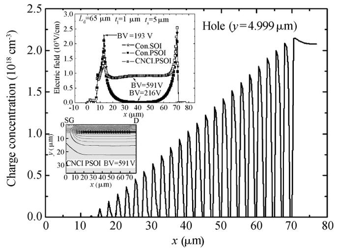
Fig. 2. Distributions of the interface holes ( $y = 4.999 \mu\text{m}$ ), the surface electric field ( $y = 0.001 \mu\text{m}$ ) and the equipotential contours for the CNCI PSOI at breakdown.
