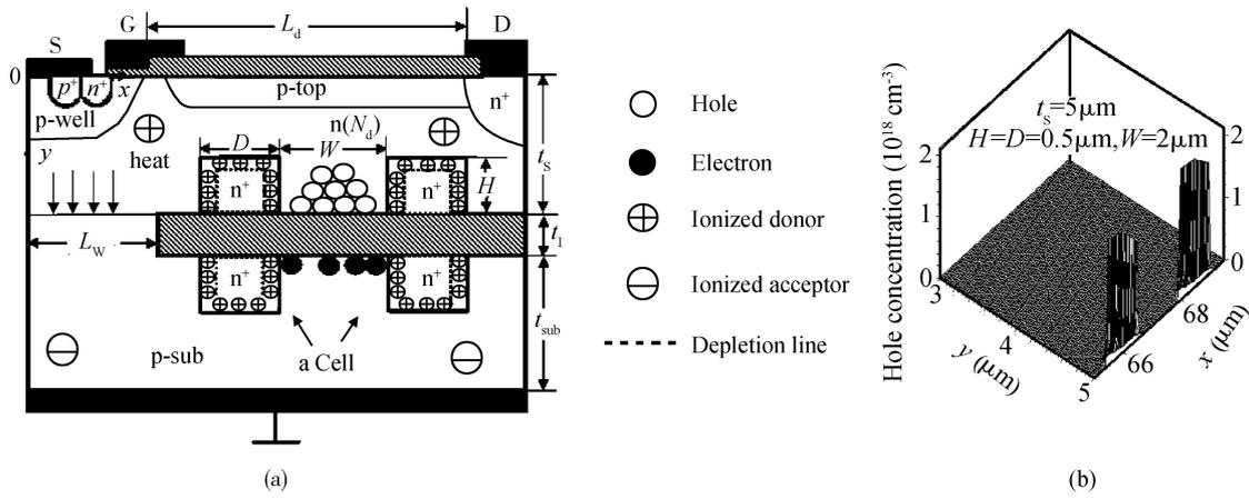
Fig. 1. Schematic cross section of CNCI PSOI LDMOS and the charges in the CNCIs. (a) Device structure. (b) Three-dimensional hole distribution in a pair of neighboring n<sup>+</sup>-regions near the drain ( $t_s = 5 \mu\text{m}$ ,  $t_1 = 1 \mu\text{m}$ ,  $H = D = 0.5 \mu\text{m}$ ,  $W = 2 \mu\text{m}$  and  $V_d = 591 \text{ V}$ ).
