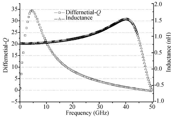
Fig. 3. Simulated  $Q$  factor and inductance of the on-chip inductor.
