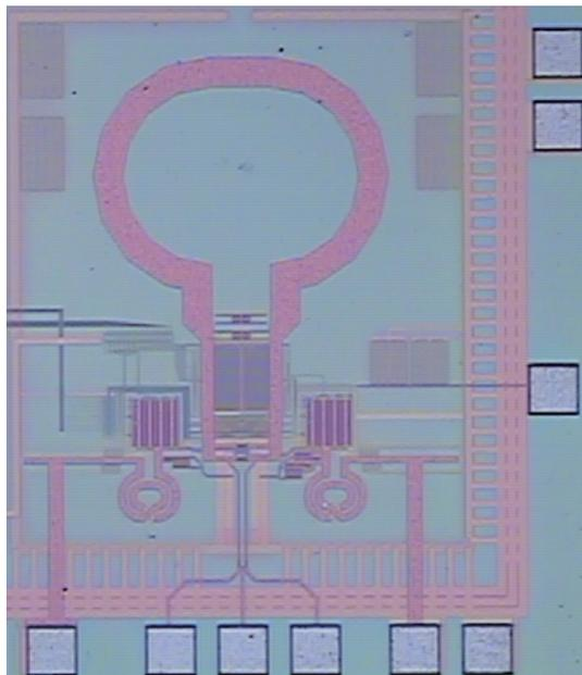
Fig. 4. Chip photograph of proposed differential LC VCO.
