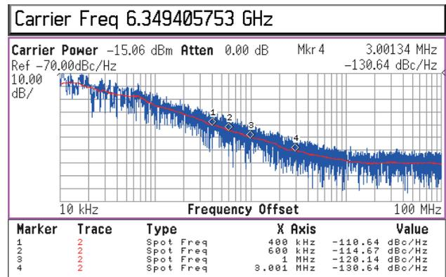
Fig. 5. Measured phase noise of proposed differential LC VCO.
