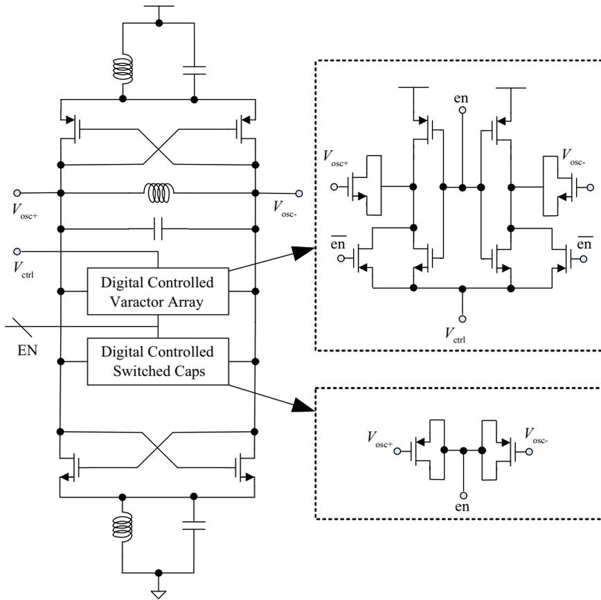
Fig. 1. Circuit diagram of the proposed differential LC VCO.
