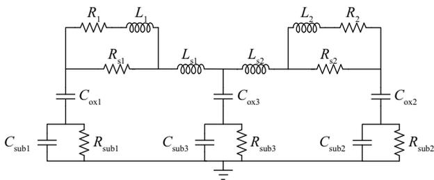
Fig. 2. Simplified double- $\pi$  equivalent circuit of a single turn spiral inductor.
