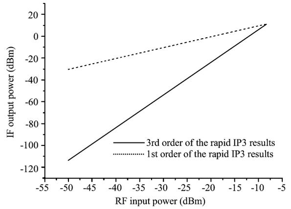
Fig. 9. Post-simulated IIP3 of the current-mode RF receiver front-end.
