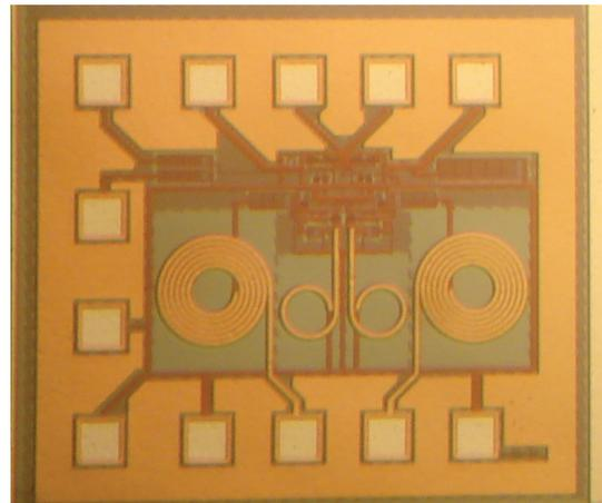
Fig. 10. Microphotograph of the current-mode RF receiver front-end.
