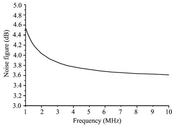
Fig. 8. Post-simulated noise of the current-mode RF receiver front-end.
