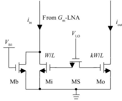
Fig. 5. Proposed switched current mirror—core of the switched current mirror current-mode mixer.
