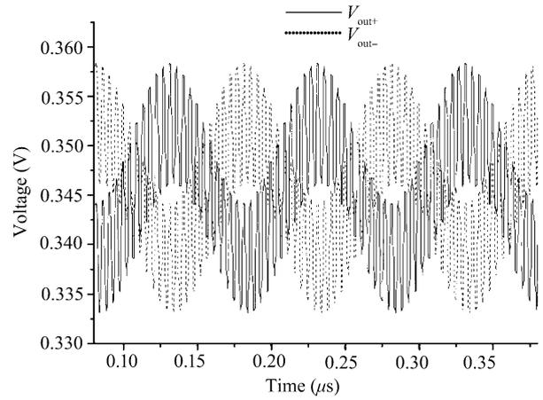
Fig. 6. Post-simulated differential output of the current-mode RF receiver front-end.
