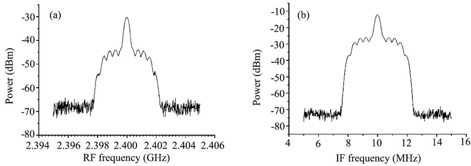
Fig. 11. Measured spectra of the (a) input and (b) output frequency.
