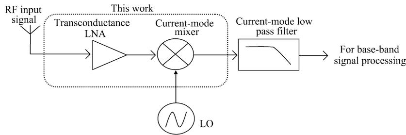
Fig. 1. Whole block diagram of current-mode RF receiver of direct conversion.
