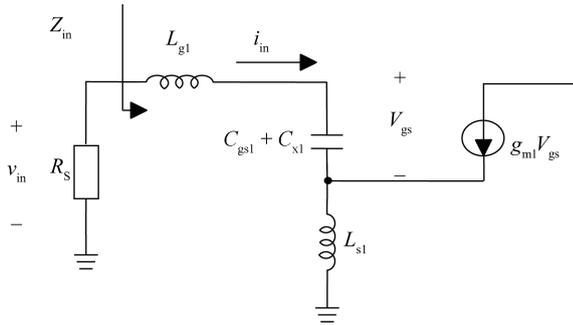
Fig. 4. Small signal equivalent circuit of the transconductance LNA's input port.
