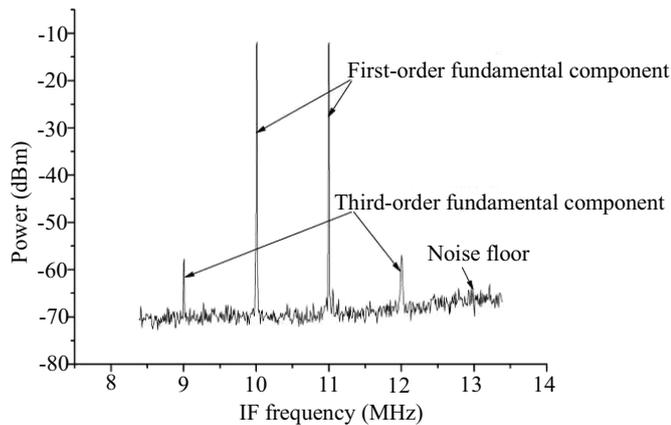
Fig. 12. Measured spectrum for calculating the IIP3 of the current-mode RF receiver front-end.
