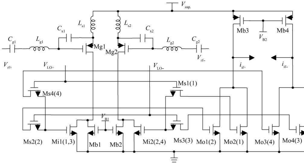
Fig. 2. Proposed low voltage current-mode RF receiver front-end circuit.
