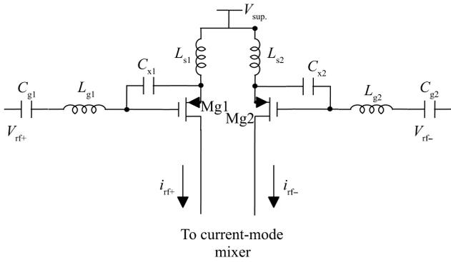
Fig. 3. Schematic diagram of the differential CMOS transconductance LNA.
