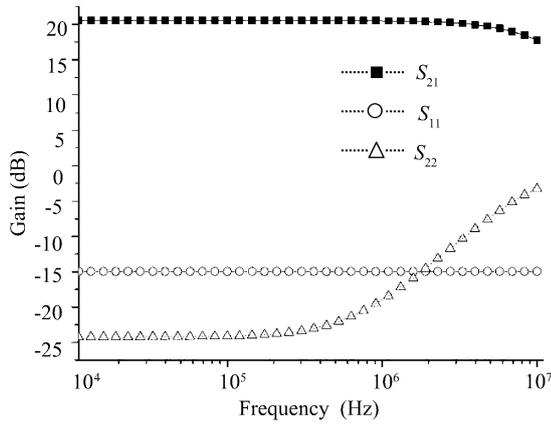
Fig. 7. Post-simulated  $S$  parameters of the current-mode RF receiver front-end.
