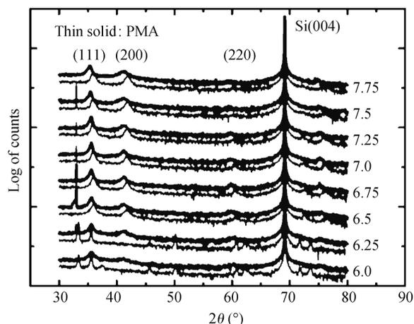
Fig. 2. Glancing angle XRD spectra of TaN films versus depositing N<sub>2</sub> flow rate: as-deposited (thick solid) and after a PMA of 900 °C/1 min in N<sub>2</sub> (thin solid).
