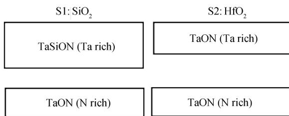
Fig. 6. Schematic diagrams of interfacial layer formation after a PMA of 900 °C/1 min in N<sub>2</sub> for S1 and S2 under Ta-rich and N-rich conditions.
