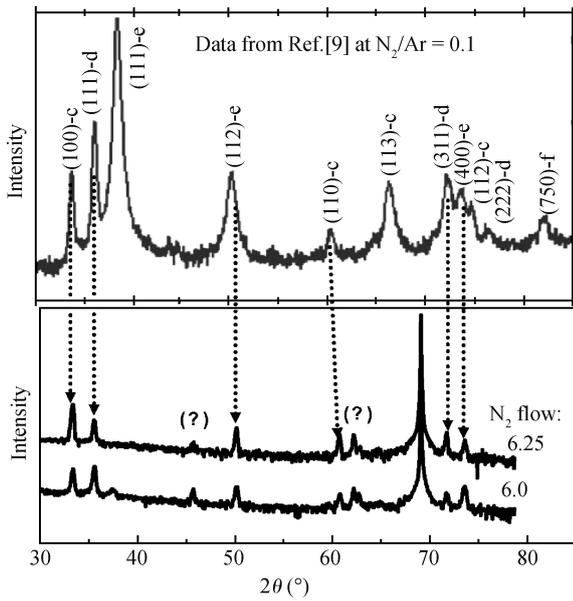
Fig. 3. Comparison of XRD spectra of TaN films ( $N_2$  flow rate: 6.0 and 6.25 sccm) after PMA with the data of Ref. [10]. The four phases in the data of Ref. [10] are: c-TaN<sub>0.8</sub> (hexagonal), d-TaN (fcc cubic), e-Ta<sub>4</sub>N (orthogonal) and f-TaN<sub>0.04</sub> (cubic).
