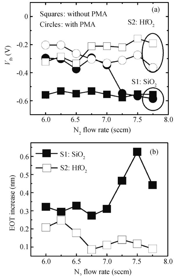
Fig. 5. TaN-gated MOS capacitors with gate stacks of S1: TaN/4 nm SiO<sub>2</sub>/p-Si (called as SiO<sub>2</sub>) and S2: TaN/5 nm HfO<sub>2</sub>/4 nm SiO<sub>2</sub>/p-Si (called as HfO<sub>2</sub>). (a)  $V_{fb}$  versus  $N_2$  flow rate for cases of without and with a PMA of 900 °C/1min in  $N_2$ . (b) EOT increase versus  $N_2$  flow rate after the PMA.
