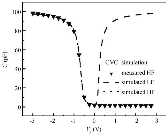
Fig. 4. Measured HF, simulated HF and LF CV curves for a capacitor with gate stack S1 and PDA-only using CVC program. The  $N_2$  flow rate was 7.25 sccm. The extracted  $V_{fb}$  and EOT are  $-0.554$  V and 3.91 nm, respectively.
