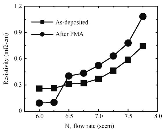
Fig. 1. Resistivity of 200 nm TaN films versus N<sub>2</sub> flow rate: as-deposited and after a PMA of 900 °C/1 min in N<sub>2</sub>.
