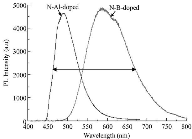
Fig. 2. Photoluminescence spectra of f-SiC epilayers.
