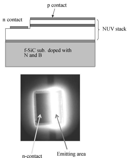
Fig. 6. Schematic diagram of warm-white LED and photograph showing the operation.
