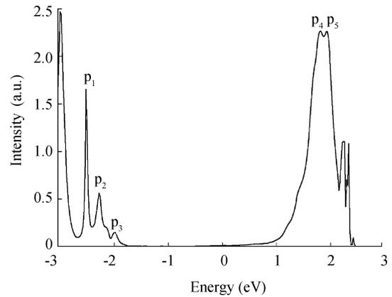
Fig. 3. Equilibrium transmission spectrum of the heterojunction.
