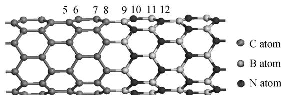
Fig. 1. An optimized (8, 0) CNT/BNNT heterojunction.
