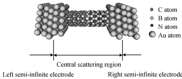
Fig. 2. A two-probe model for the heterojunction coupled to Au electrodes.
