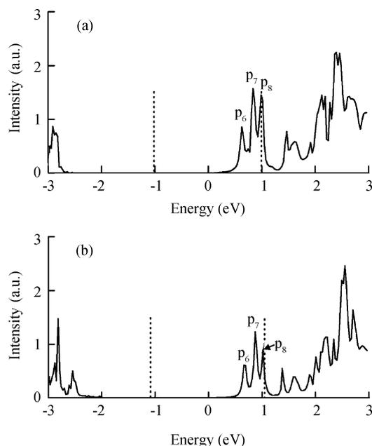
Fig. 6. Transmission spectra of the heterojunction under bias of (a)  $V = +2.0$  V and (b)  $V = +2.2$  V.
