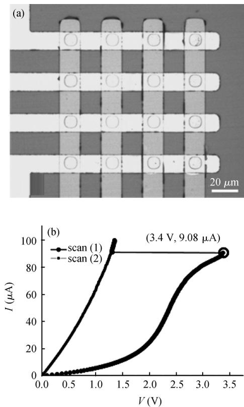
Fig. 6. (a) Microscope image of a vertical PCRAM device with an ELD Ni plug. (b)  $I$ - $V$  characteristics of a vertical PCRAM device with an ELD Ni plug.
