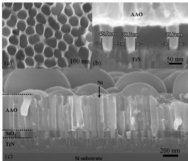
Fig. 3. (a) Top view SEM image of an ELD Ni nanoplug on TiN substrate. (b) Cross-sectional SEM image of an ELD Ni nanoplug on TiN substrate. (c) Full view cross-sectional SEM image of an ELD Ni nanoplug on TiN substrate.
