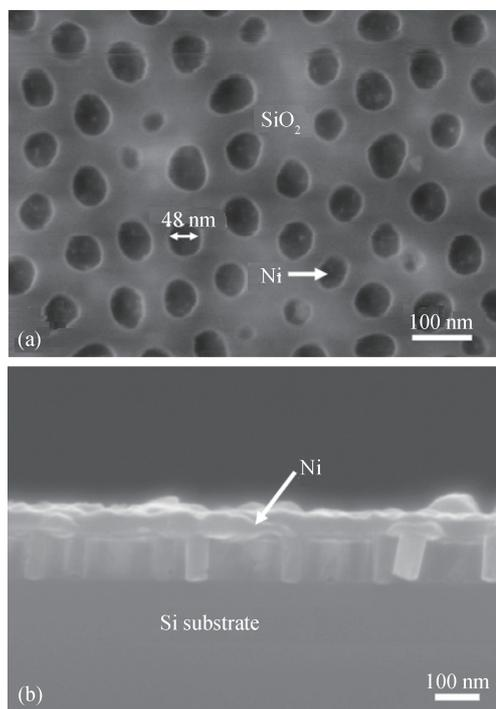
Fig. 2. (a) Top view SEM image of an ELD Ni nanoplug on Si substrate. (b) Cross-sectional SEM image of an ELD Ni nanoplug on Si substrate.
