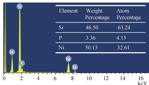
Fig. 5. EDX results of an ELD Ni nanoplug on Si substrate.
