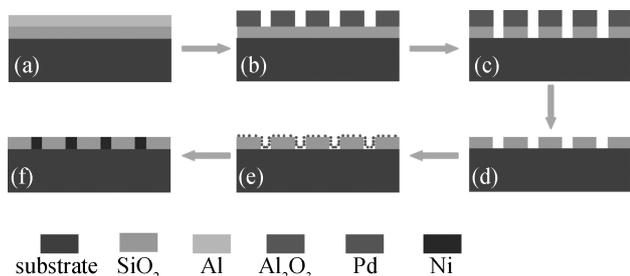
Fig. 1. Schematic process for metal nanoplug fabrication. (a) Al and SiO<sub>2</sub> deposition, the substrate can be Si, W/Si or TiN/Si. (b) Formation of AAO template by two-step anodization. (c) Dry etching of SiO<sub>2</sub>. (d) Chemical dissolution of AAO template. (e) Activation of the surface before deposition and (f) ELD Ni.
