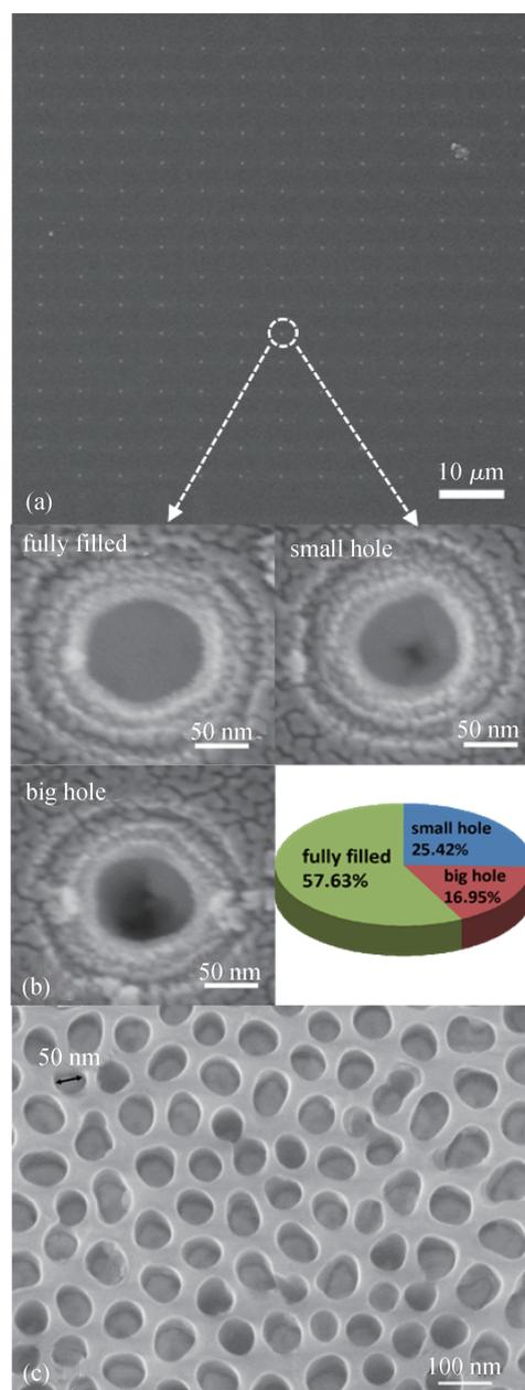
Fig. 4. (a) Top view SEM image of an ELD Ni nanoplug on W substrate in a test structure with a via size of 90 nm. (b) Top view SEM images and statistical chart of different filling results. (c) Top view SEM image of an ELD Ni nanoplug through an AAO template on W substrate. A thin layer of gold was sputtered on the surface before SEM observing in (a) and (b).
