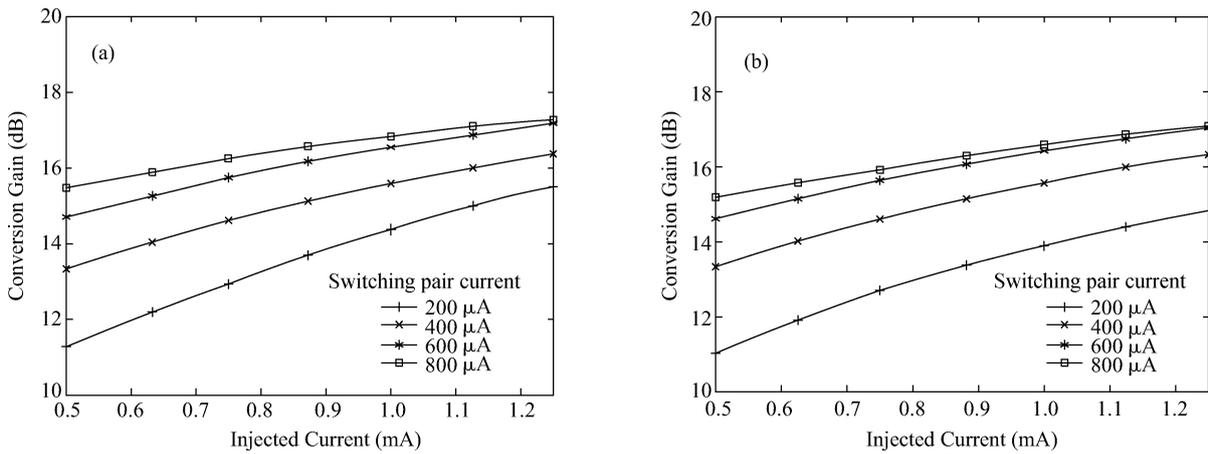
Fig. 7. Simulated conversion gain with fixed tail current but increasing ratio between injection bypass current and switching pair current of (a) 1.27 GHz-RF 50 MHz-IF operation and (b) 1.575 GHz-RF 2 MHz-IF operation.
