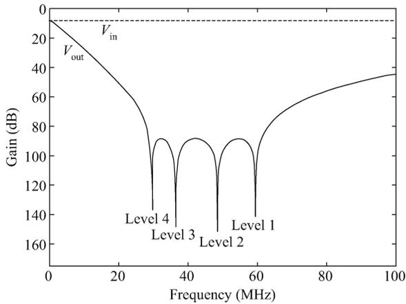
Fig. 13. Response of proposed four-stage RC polyphase filter.
