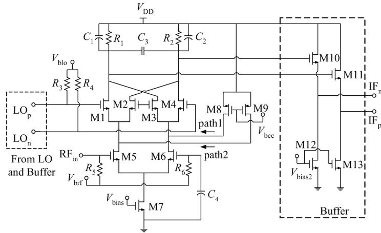
Fig. 6. Schematic of proposed down-conversion mixer.
