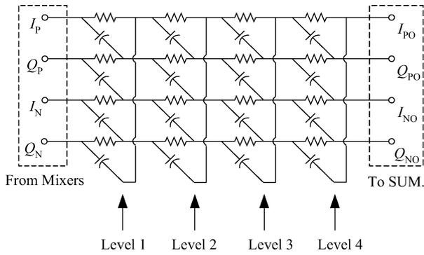
Fig. 12. Schematic of proposed polyphase filter.
