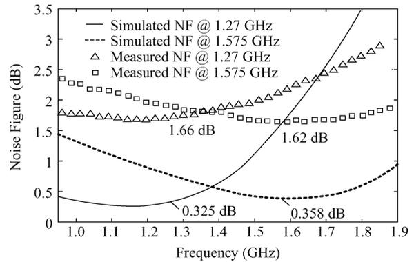
Fig. 4. Simulated and measured noise figure of 1.27 GHz operation and 1.575 GHz operation.
