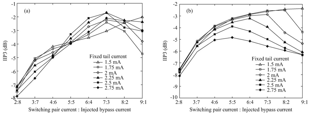
Fig. 11. Simulated IIP3 with fixed tail current but increasing ratio between inject bypass current and switching pair current of (a) 1.27 GHz-RF 50 MHz-IF operation and (b) 1.575 GHz-RF 2 MHz-IF operation.
