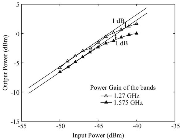
Fig. 17. Power gain and the  $P_{1dB}$  of the frontend blocks.
