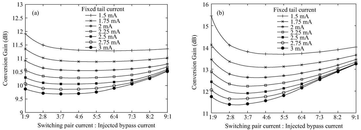
Fig. 10. Simulated conversion gain with fixed tail current but increasing ratio between inject bypass current and switching pair current of (a) 1.27 GHz-RF 50MHz-IF operation and (b) 1.575 GHz-RF 2 MHz-IF operation.
