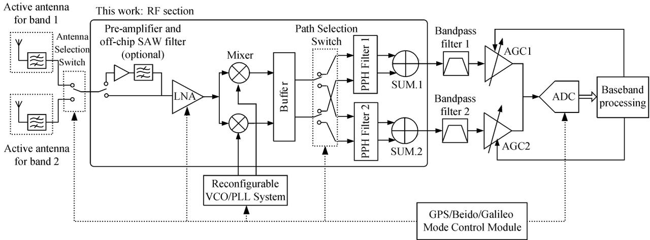
Fig. 1. Block diagram of proposed multi-band receiver architecture.
