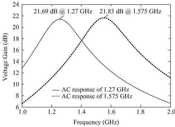
Fig. 5. Voltage gain of different frequency bands.
