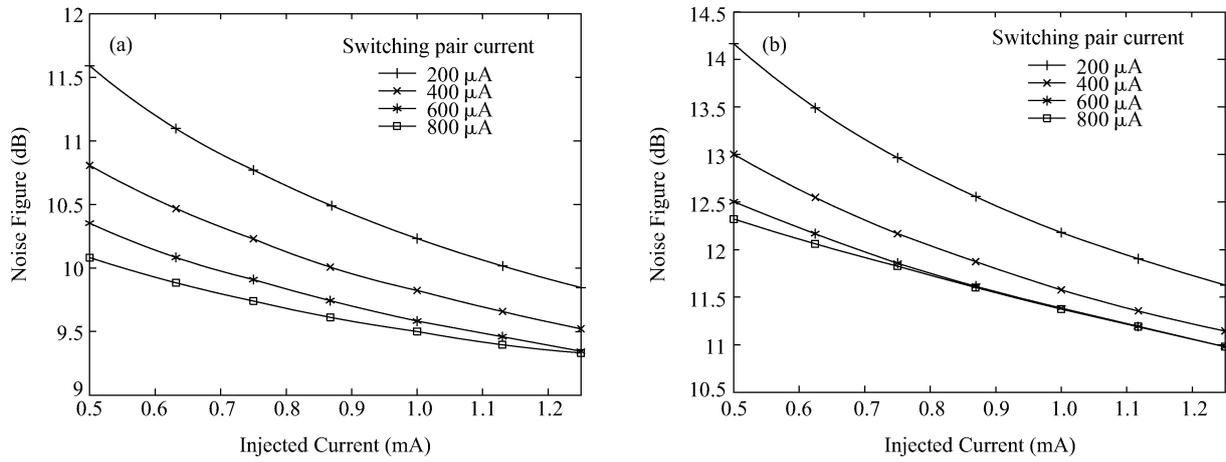
Fig. 9. Simulated noise figure with fixed switching pair current but increasing inject bypass current of (a) 1.27 GHz-RF 50 MHz-IF operation and (b) 1.575 GHz-RF 2 MHz-IF operation.
