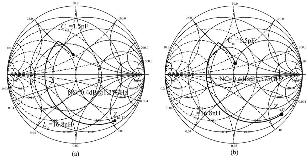
Fig. 3. Input impedance matching in the Smith chart for (a) 1.27 GHz operation and (b) 1.575 GHz operation.
