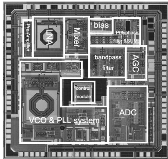
Fig. 15. Micrograph of the complete receiver chip.
