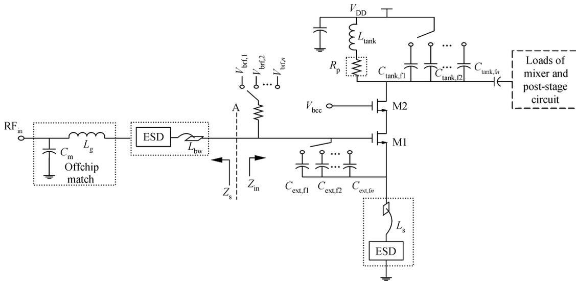
Fig. 2. Schematic of the proposed LNA.
