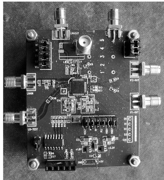
Fig. 16. Test board with the chip.
