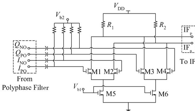
Fig. 14. Schematic of the proposed summing circuit.
