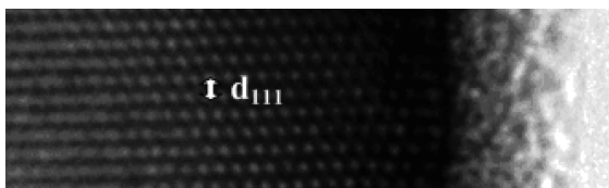
Fig. 8. High-resolution TEM image of the nanowire with a diameter of 228 nm.
