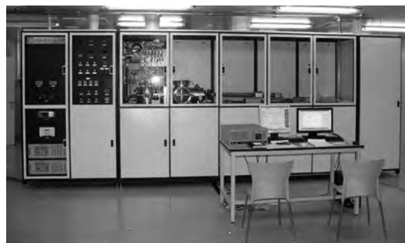
Fig. 1. Overall view of the MOCVD system.
