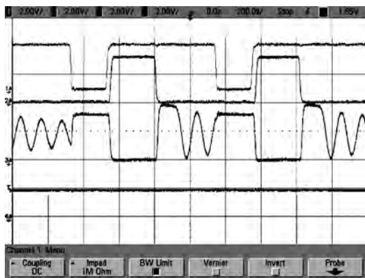
Fig. 15. Waveforms when DCM control is on (from top to bottom: V_{gpi} , V_{gni} , V_{sw} , V_{out} ).
