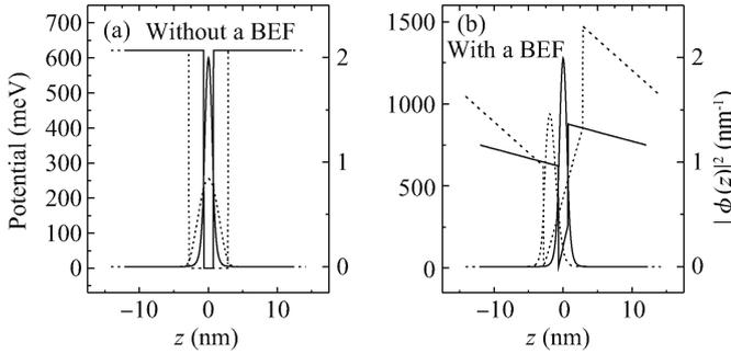
Fig. 2. Schematic potential profiles and squared wave functions of electrons at ground states for WZ GaN/AlN QWs (a) without and (b) with a BEF corresponding to  $d = 0.5a_0$  (solid lines) and  $d = 2a_0$  (dashed lines). The left (right) perpendicular axes are in units of meV ( $\text{nm}^{-1}$ ).
