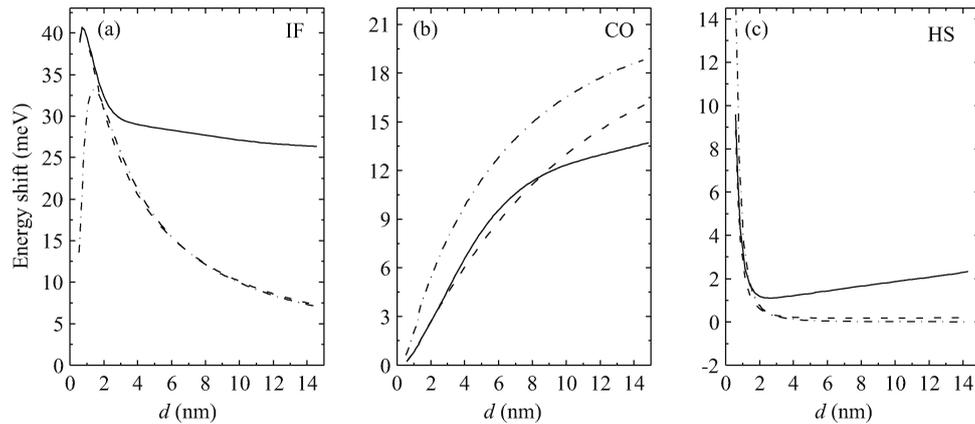
Fig. 4. Polaron energy shifts (a)  $\Delta E_{IF}$ , (b)  $\Delta E_{CO}$ , and (c)  $\Delta E_{HS}$  as functions of the well width  $d$  for GaN/AlN WZ QWs with (solid lines) and without (dash lines) a BEF, and for ZB QWs (dash-dotted lines).
