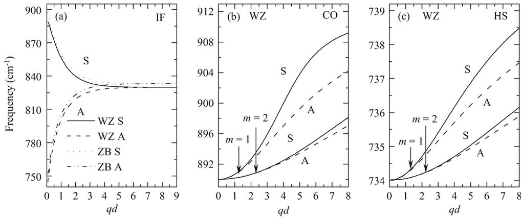
Fig. 3. Dispersion relations of (a) IF, (b) CO and (c) HS phonon modes in GaN/AlN WZ QWs. The symmetric and antisymmetric modes are denoted as S (solid lines) and A (dashed lines), respectively. The symmetric (dotted line) and antisymmetric (dash-dotted line) IF modes in ZB QWs are also plotted in (a).
