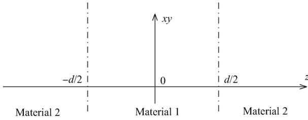
Fig. 1. A schematic geometry of GaN/AlN QWs.
