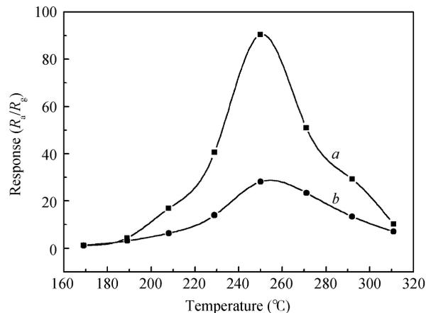
Fig. 3. Response of (a) our flower-like ZnO products and (b) sword-like ZnO nanorod bundles to 500 ppm ethanol at different operating temperatures, respectively.
