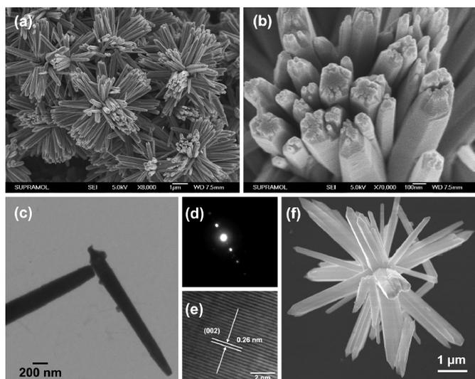
Fig. 2. Morphological and structural characterizations of the ZnO products. (a) and (b) different magnification FESEM images. (c) TEM image. (d) SAED pattern and (e) HRTEM image of part of a ZnO nanorod. (f) The FESEM image of the sword-like ZnO nanorod bundles prepared with CTAB.
