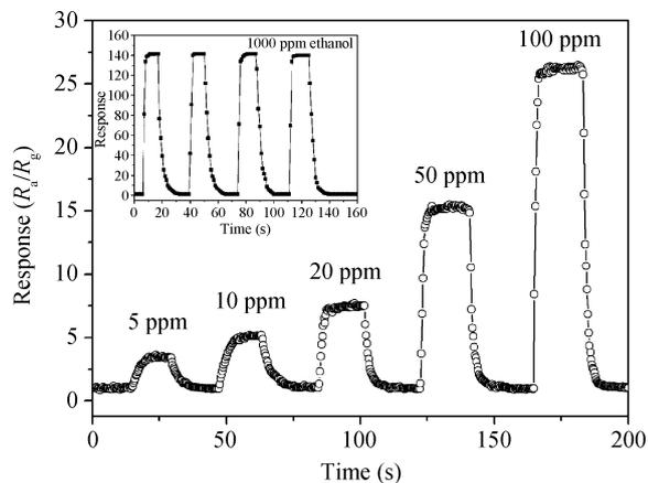
Fig. 4. Response of the flower-like ZnO nanostructures to ethanol of various concentrations at 250 °C. The inset shows the consistent response and recovery throughout the four cyclic tests.
