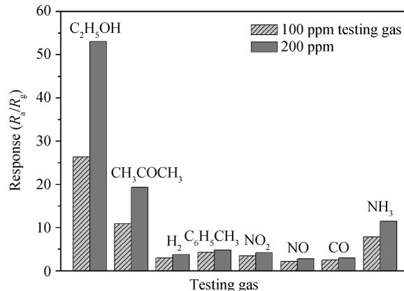
Fig. 6. Response of the flower-like ZnO nanostructures to various test gases.
