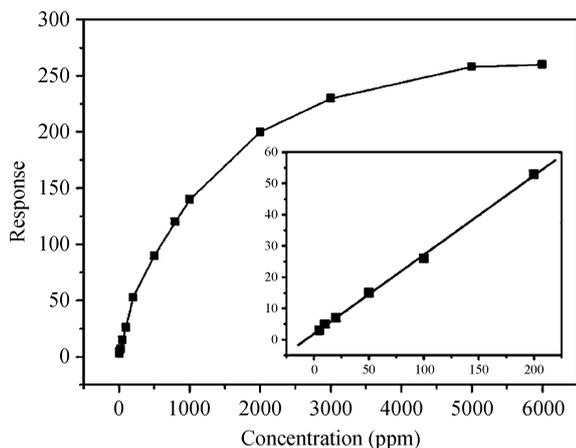
Fig. 5. Response of the flower-like ZnO nanostructures versus ethanol concentration. The inset shows a linear dependence of the response on the ethanol concentration in the range of 1–200 ppm.
