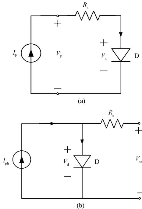
Fig. 5. Equivalent circuits when LED is (a) electrical injected and (b) photo-excited (open-circuit).
