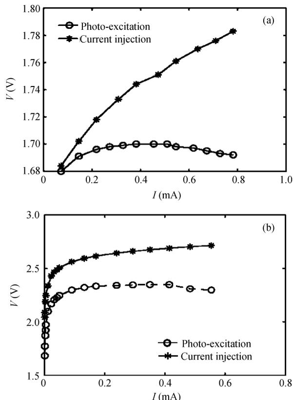
Fig. 3. *I*–*V* curves of (a) a red AlGaInP and (b) a green InGaN LED under photo-excitation and current injection. For photo-excitation, the horizontal axis indicates the photo-generated current and the vertical axis indicates the open-circuit voltage. For current injection, the horizontal axis indicates the forward drive current and the vertical axis indicates the forward-bias voltage.
