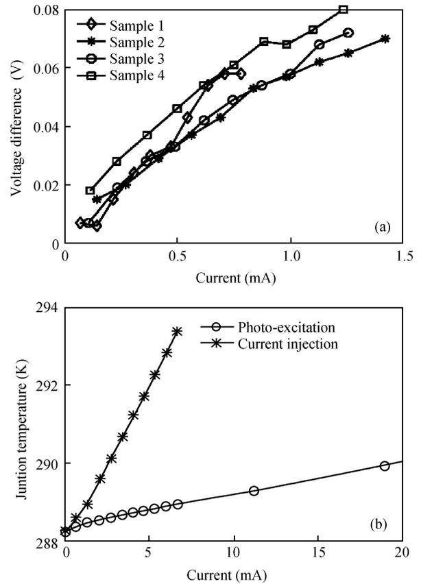
Fig. 6. (a) Dependences of the voltage differences between these two injection ways on the injection currents. (b) Dependences of the junction temperatures on the injection currents in a red AlGaInP LED.
