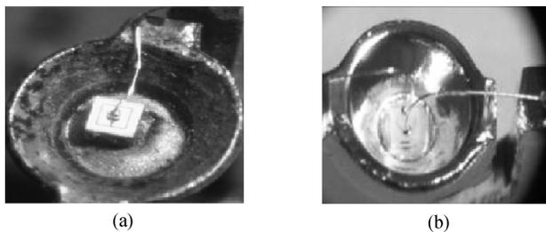
Fig. 1. Top views of (a) a red AlGaInP and (b) a green InGaN LED chip bonded in a lead frame.
