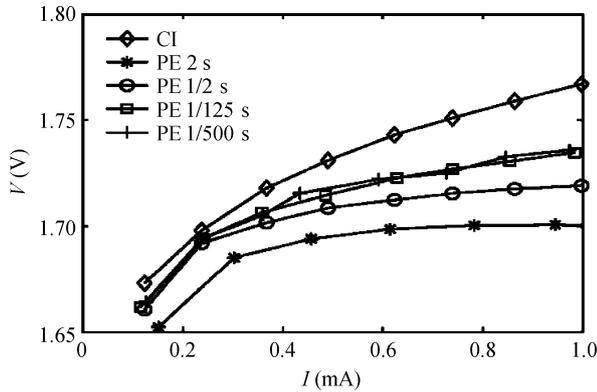
Fig. 7.  $I$ - $V$  characteristics under pulsed light excitation, as well as those under current injection.
