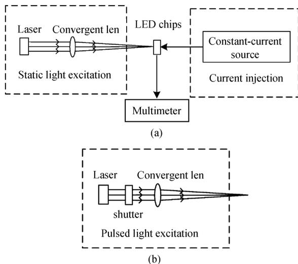
Fig. 2. Schematic of measurement of the current–voltage characteristics under (a) static light excitation, current injection and (b) pulsed light excitation.
