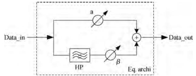
Fig. 3. Block diagram of a conventional equalizer.
