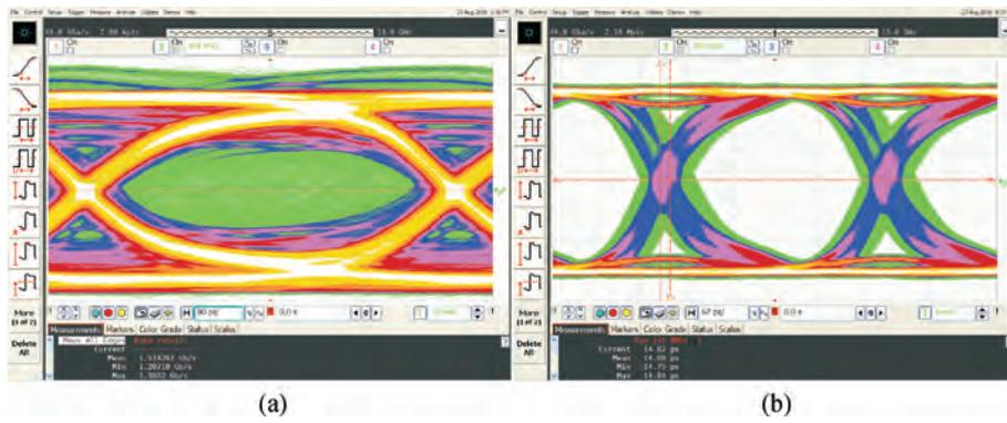
Fig. 15. Equalizer results for a 1.5 Gbps data rate. (a) Before equalization. (b) After equalization.
