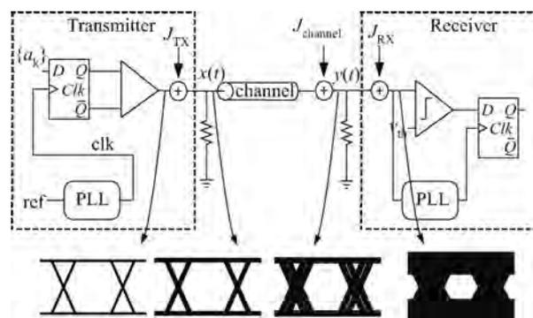
Fig. 1. Schematic of Serdes architecture.
