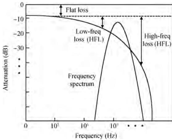
Fig. 2. Attenuation characteristic of the low-pass channel.
