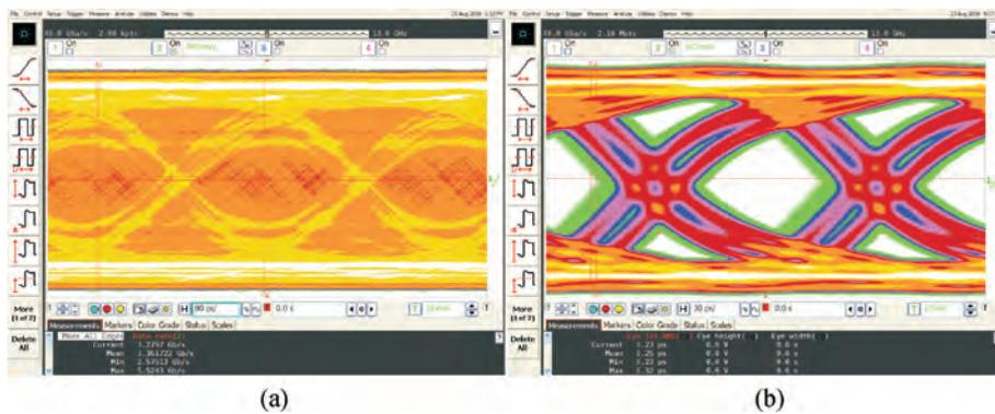
Fig. 18. Equalizer results for a 3.3 Gbps data rate. (a) Before equalization. (b) After equalization.
