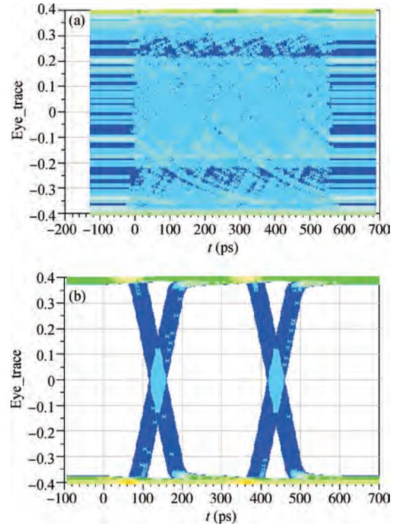
Fig. 11. Simulation result of overall topology (a) before equalizer and (b) after equalizer.
