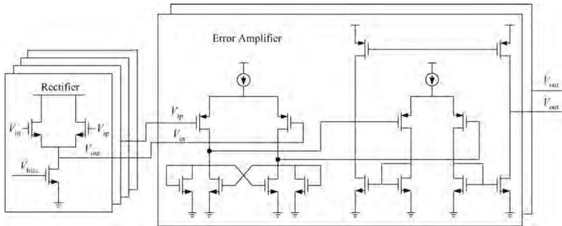
Fig. 9. Topologies of the rectifier and the error amplifier.
