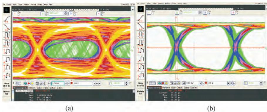
Fig. 14. Equalizer results for a 1 Gbps data rate. (a) Before equalization. (b) After equalization.
