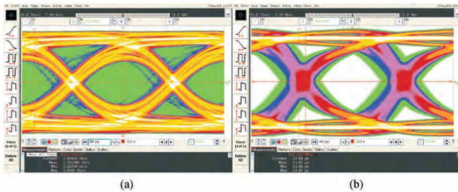
Fig. 17. Equalizer results for a 2.5 Gbps data rate. (a) Before equalization. (b) After equalization.
