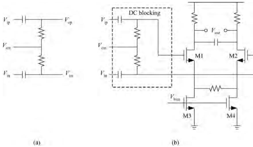
Fig. 8. (a) High-pass filter. (b) Active low-pass filter.
