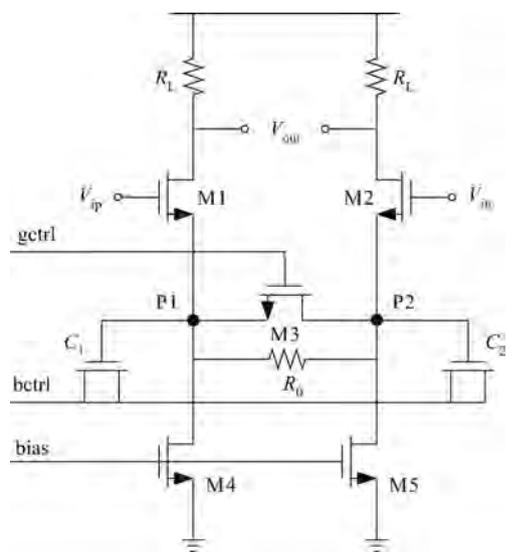
Fig. 6. Topology of the implemented analog equalizer.
