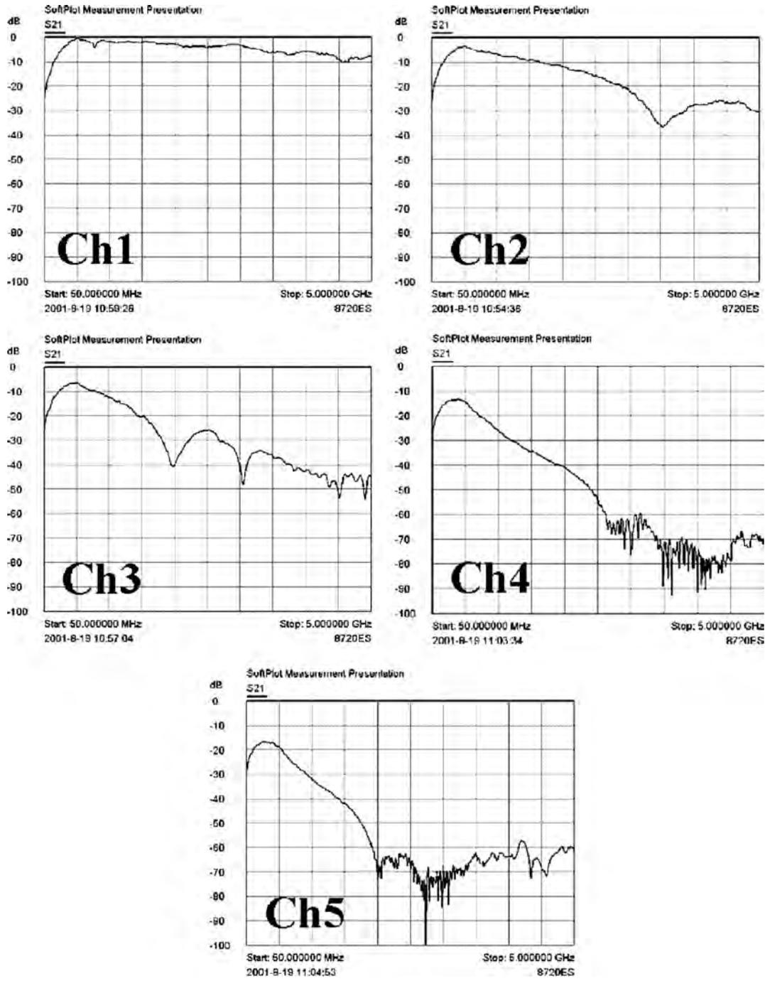
Fig. 13. Measurement of the  $S$  parameter of channel loss.
