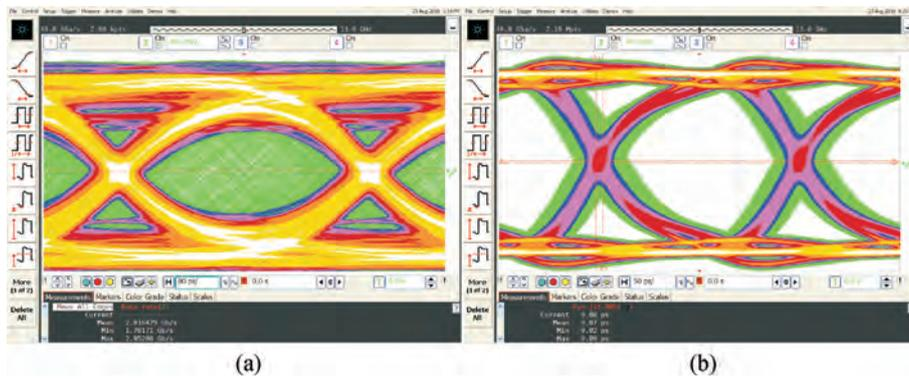
Fig. 16. Equalizer results for a 2 Gbps data rate. (a) Before equalization. (b) After equalization.
