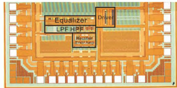
Fig. 12. Photomicrograph of prototype chip.
