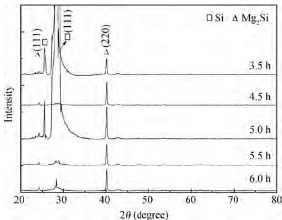
Fig. 4. XRD patterns of  $\text{Mg}_2\text{Si}$  films annealed at  $400\text{ }^\circ\text{C}$  for various annealing times.
