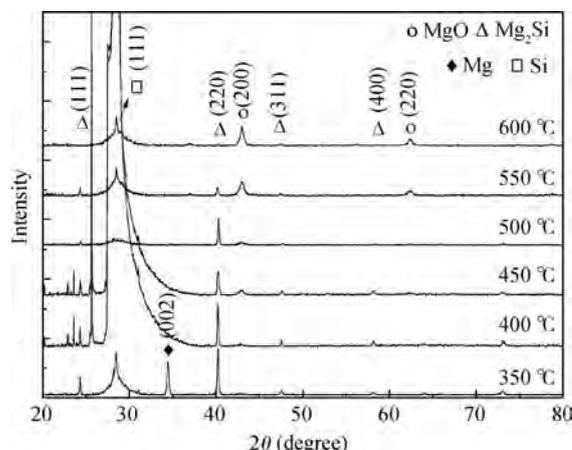
Fig. 2. XRD patterns of  $\text{Mg}_2\text{Si}$  films annealed at various annealing temperatures for 380-nm-thick magnesium film on silicon substrates.
