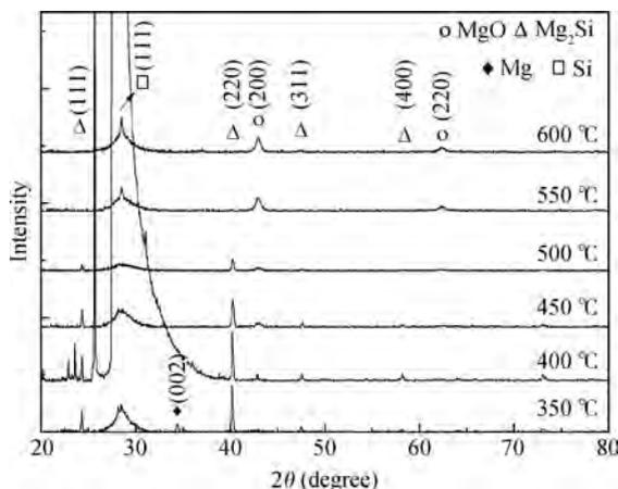
Fig. 1. XRD patterns of  $\text{Mg}_2\text{Si}$  films annealed at various annealing temperatures for 280-nm-thick magnesium film on silicon substrates.
