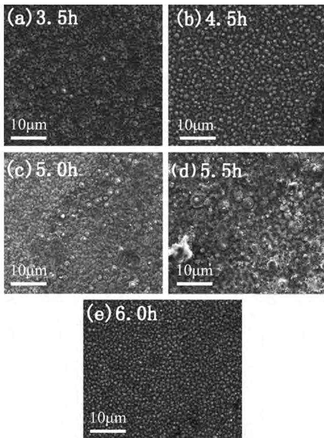
Fig. 6. SEM images of the samples annealed at 400 °C for various annealing times.
