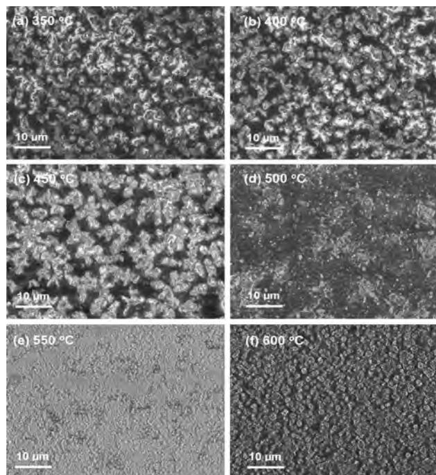
Fig. 5. SEM images of the samples annealed at various annealing temperatures for 5 h.
