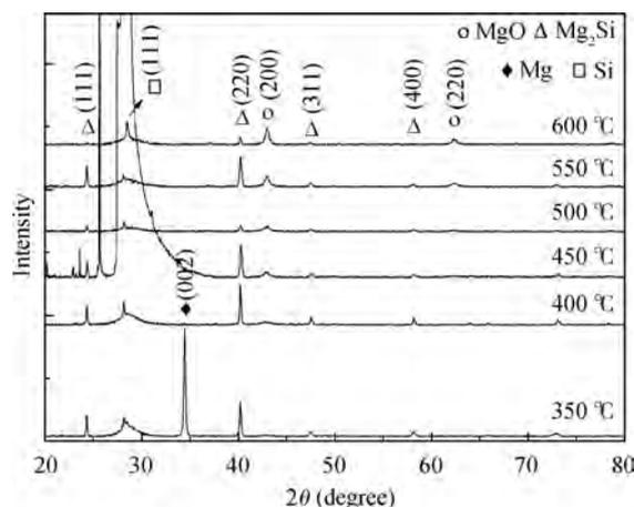
Fig. 3. XRD patterns of  $\text{Mg}_2\text{Si}$  films annealed at various annealing temperatures for 480-nm-thick magnesium film on silicon substrates.
