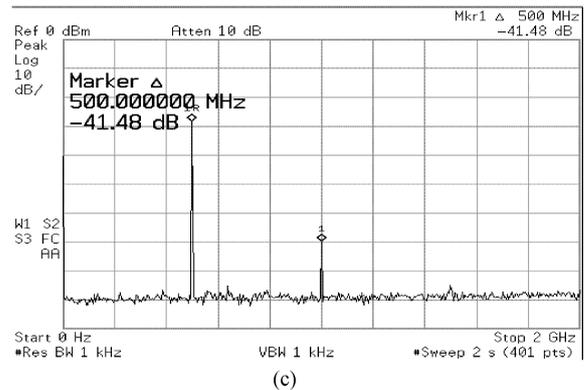
Fig. 6. Output spectra. (a)  $f_{out} = 199.5 \text{ MHz @ } 1.2 \text{ GHz}$ . (b)  $f_{out} = 19.95 \text{ MHz @ } 1.2 \text{ GHz}$ . (c)  $f_{out} = 500 \text{ MHz @ } 1.2 \text{ GHz}$ .
