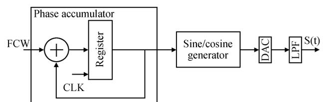
Fig. 1. Schematic of a traditional DDFS system.
