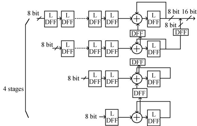
Fig. 3. Architecture of the pipelined accumulator in this work.
