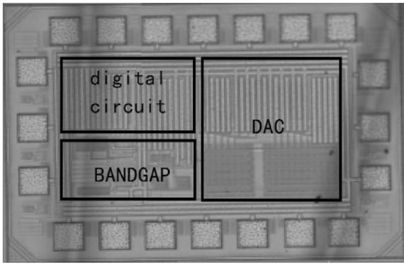
Fig. 5. Micro-photo of the MUX-DDFS chip.
