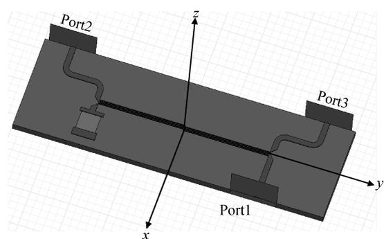
Fig. 1. Lange coupler's three-dimensional model of Ansoft HFSS.
