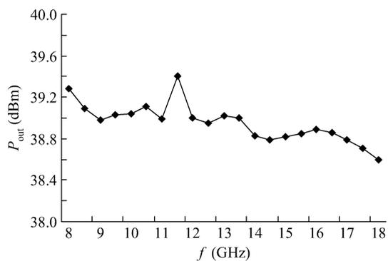
Fig. 8. Saturated output power ( $V_d = 8$  V,  $P_{in} = 25$  dBm).
