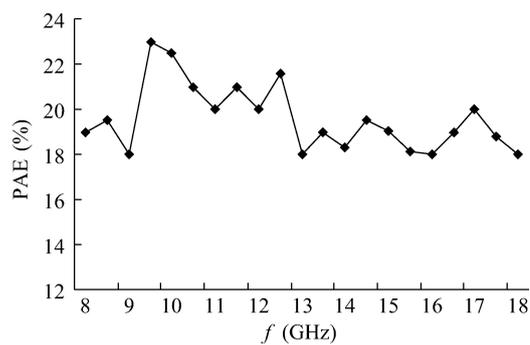
Fig. 9. Power-added efficiency ( $V_d = 8$  V,  $P_{in} = 25$  dBm).
