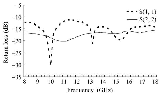
Fig. 12. The measured small-signal return loss of the amplifier.
