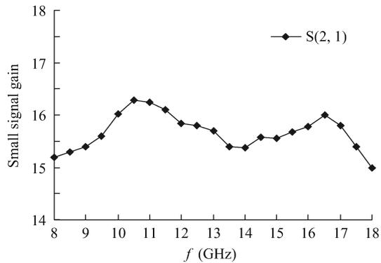
Fig. 11. The measured small signal gain ( $P_{in} = 18$  dBm).
