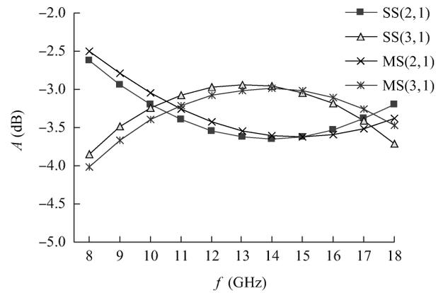
Fig. 4. Simulation and measurement results of amplitude imbalance.
